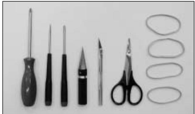
Screw Drivers, Lexan Body Reamer, Hobby Knife, Lexan Scissors, Rubber Bands.
