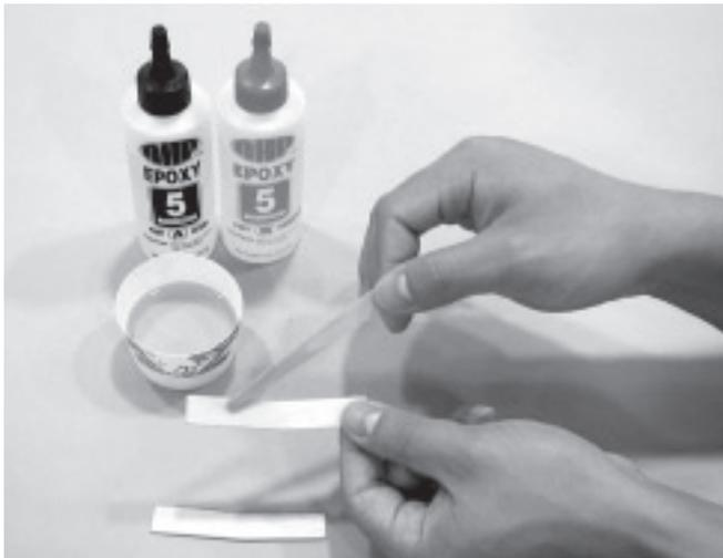
**2.** Locate two dihedral plywood wing joiners. Glue two wing joiners together with 5-minute Epoxy.
