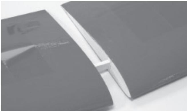
**5.** Lightly coat epoxy on all sides of the other half of the wing joiner (exposed part) and the exposed balsa inner edges of both wing panels (called the wing root). Slide the wing halves together, ensuring that they are accurately aligned. Firmly press the halves together and wipe off any excess epoxy. Let the epoxy cure while holding the wing together in proper alignment.
