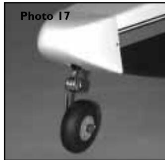
The nosegear is configured as shown in the above photo. The linkage is a piece of music wire that goes through an inner nyrod that has already been installed in the fuselage. Use a "Z" bend at the steering arm end (center hole in the arm). With the music wire linkage installed, mount the nosegear bracket to the nose of the plane using the 3x12mm self tap screws furnished (drill 1/16" pilot holes.) The bottom of the nose gear bracket should line up with the bottom of the nose of the plane.
