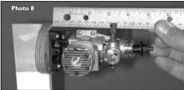
Position your engine on the engine mount (note that the mount's beam width is adjustable to accommodate your engine). Locate the engine on the mount so the front of the prop's thrust washer is  $4\frac{1}{4}$ " from the front surface of the firewall. Double check that this set-up gives you  $\frac{1}{8}$ "- $\frac{1}{4}$ " of spinner clearance from the front of the engine pod. Mark then drill pilot holes using a  $\frac{3}{32}$ " bit. Mount your engine using the four M3 X 15mm screws.
