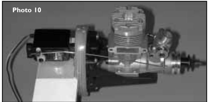
Remove the front and rear pod halves. The throttle servo is mounted on the right side of the engine pylon behind the firewall using servo tape. The throttle linkage consists of a length of music wire with a "Z" bend on the throttle arm end and an EZ connect on the servo arm end. The servo cable goes into the slot that is machined in the rear of the engine pylon.
