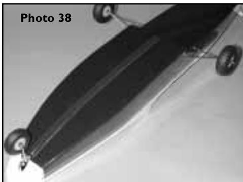
Turn the fuselage over and use "Zap-a-dap-a-goo" to fasten the formed plastic keel to the middle of the bottom of the fuselage, lining the rear edge up with the rear edge of the "step".
