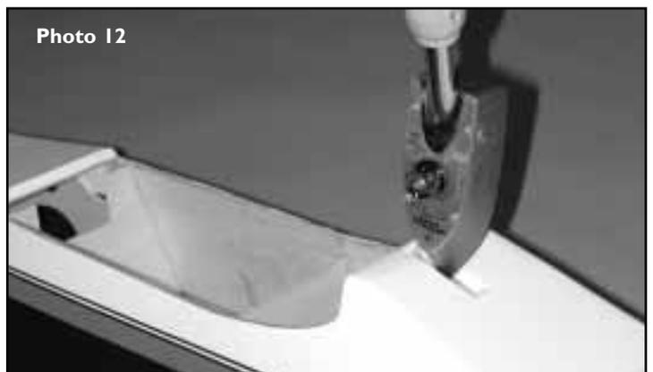
To prevent damage, have a piece of foam over your work surface to rest the hull of the fuselage upon as you work on it. Cut away the covering film that is over the slot for the engine pylon, leaving  $\frac{1}{4}$ " excess all along the slot. Cut the film diagonally to each corner and then use a heat sealing iron to seal the edges along the inside surfaces of the slot.
