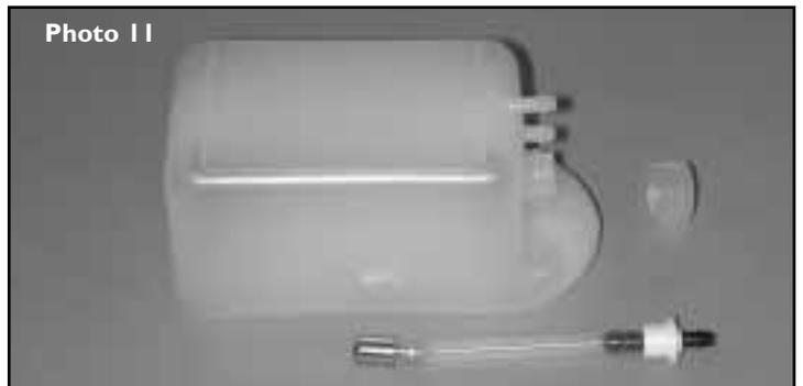
Assemble the fuel tank as shown. The fuel tank is housed in the rear engine pod and held in place with lightly wrapped foam rubber.
