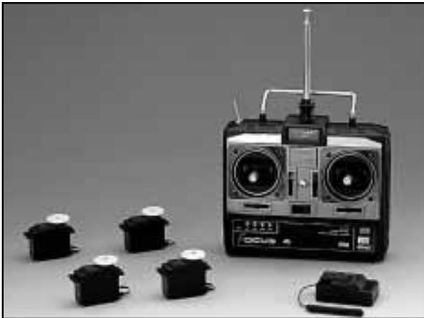
**Radio** - A 4-channel radio with four standard servos is required.
