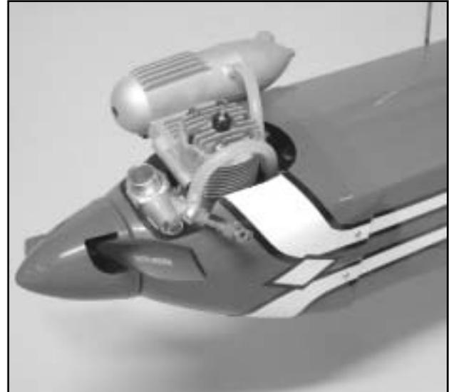
□ Trim the rear of the cowl to remove the molding flange. Make cutouts as needed to clear the prop shaft, cylinder head, carb, and muffler. A sanding wheel on a Dremel tool is handy for this.
