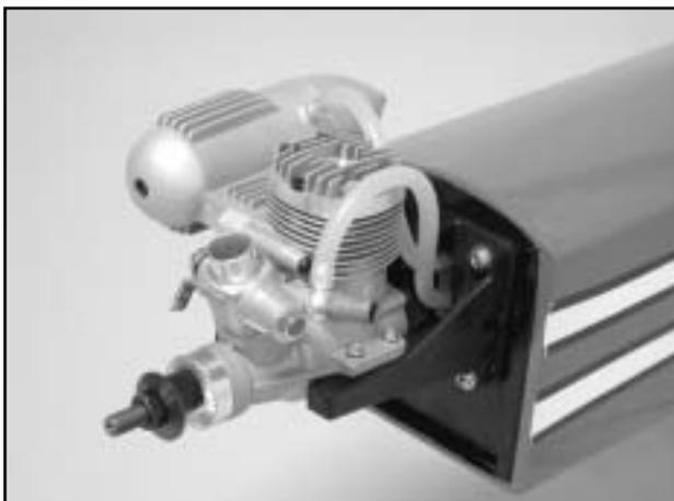
□ Slide the fuel tank (cap end first) into the front of the fuselage, threading the fuel lines through the oblong hole in the firewall. The tubing coming from the tank's fuel outlet (center) goes to the carb and the tubing from the vent (upper) goes to the muffler's pressure fitting. Trim the length as needed. Wedge some pieces of foam rubber or "bubble wrap" (not furnished) beside and on top of the tank to gently hold it in place.
