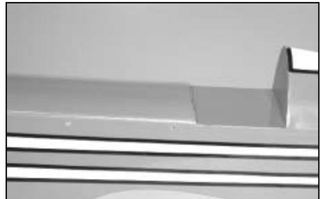
□ Locate the holes in the side of the fuselage for the cabane struts and cut away the covering material that covers them.
