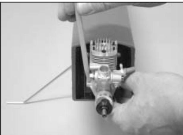
❑ Set the engine on the mount and adjust the beams so they are almost touching both sides of the engine crankcase and are centered in relation to the engine mount back plate. Now position the engine so that the front of the thrust washer is approximately 4-1/4" from the fire wall. Mark the hole locations for the engine mounting screws in the engine mount beams.
