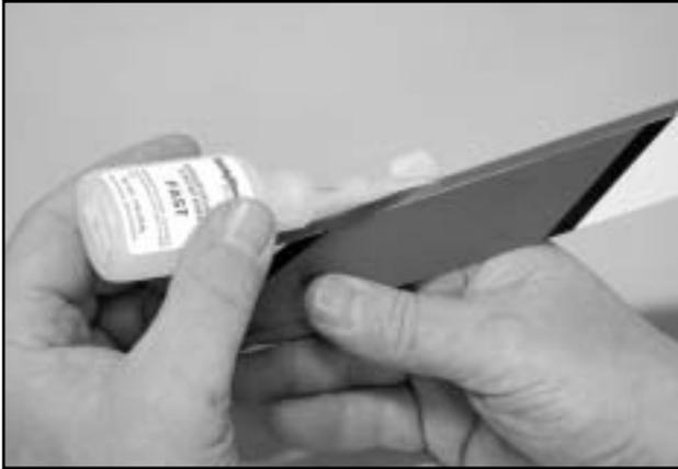
❑ To hinge the ailerons, remove the clear tape that hold the ailerons in place, if necessary. Pull the aileron off the wing, revealing the hinges. Center these hinges in their slots in the AILERON and secure them with THIN CA, letting it wick into the joint. Glue both surfaces of the hinge.
