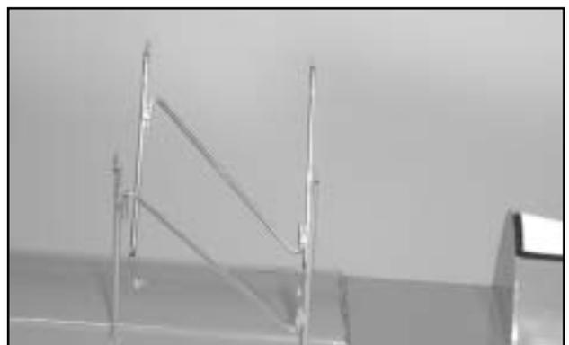
□ Insert the two preformed Cabane Struts in the holes as shown. As you look at them, they should form the letter "N". You may have to run a 1/8" drill bit in the holes to ease insertion.
