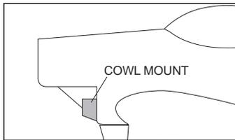
Locate two cowl mounts, epoxy them in place as diagram.
