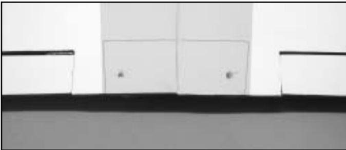
▢ Remove the plate and drill 5/16" holes in the wing for the wing bolts. Score along your marks and remove the covering. Glue the reinforcement plate in place.
