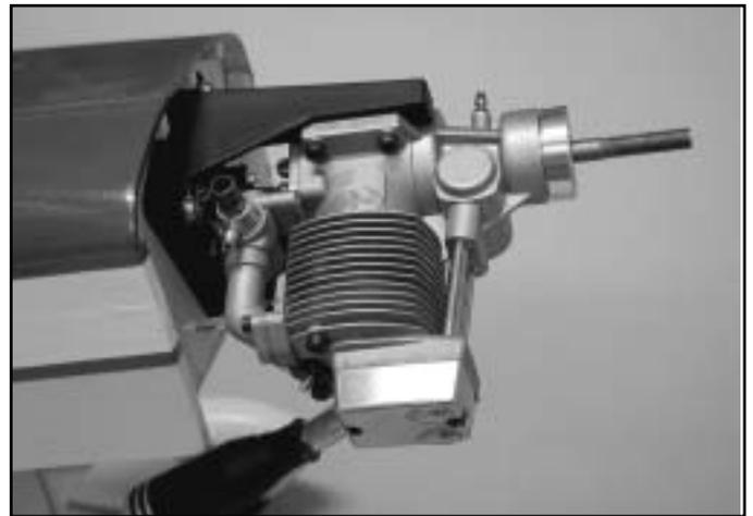
□ Attach the engine to the throttle pushrod and mount the engine in place using the four 3 x 15mm self tapping screws.
