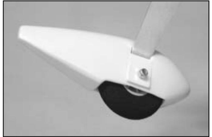
□ Locate the two wheel pants and remove the wheel opening area with an utility knife. Next, remove the small area on the inside of each wheel pant for the landing gear to set inside the wheel pant. Locate the twin axle bolts and two 4mm nuts and locknuts. Next, assemble the wheels and wheel pants onto the landing gear as shown in the picture
