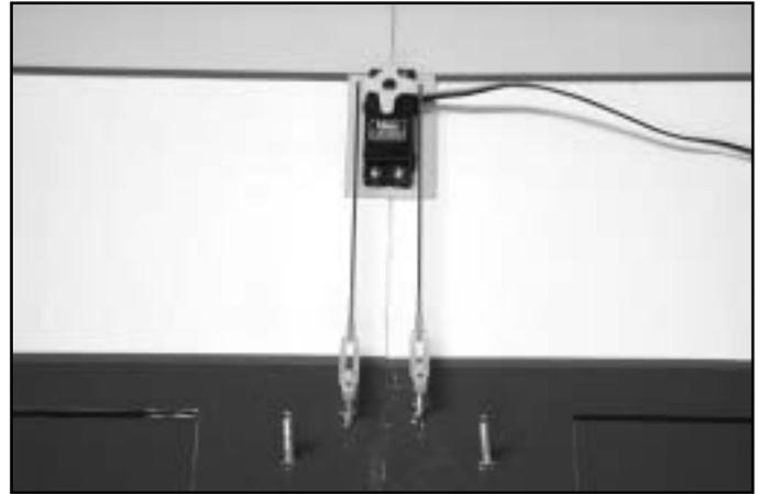
▢ Mount the servo to the wing and install the aileron linkage.
