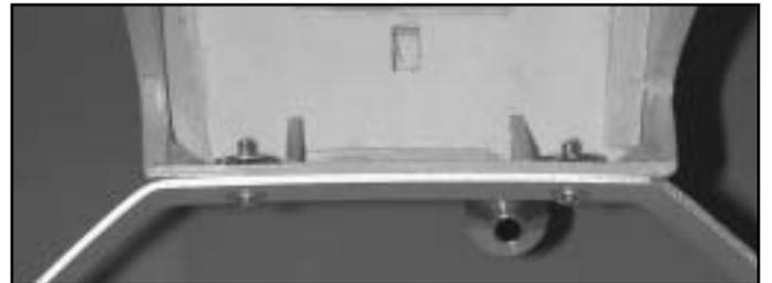
□ Attach the Main Gear to the fuselage with two 3mm bolts and blind nuts furnished.
