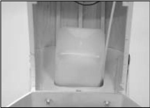
▢ Place the fuel tank in the fuselage with the fill and vent lines going through the slot provided in the firewall. Slide the tank forward into the cutout provided in the former.
