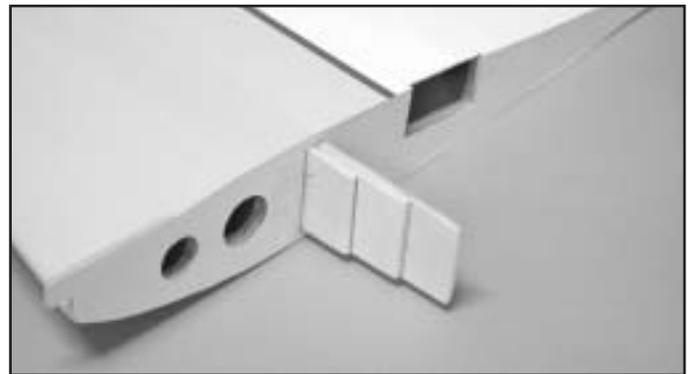
□ Epoxy the completed wing joiner to the right wing with 5 minute epoxy and let dry.
