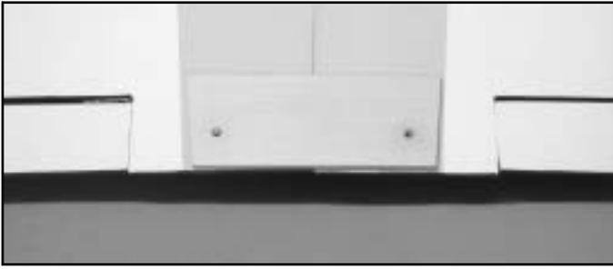
▢ Trial fit wing to fuse. With the wing in place on the fuse, place the plywood wing bolt reinforcement plate on the trailing edge of the wing and draw a line around the plate. Also use the plate as a guide to mark the two wing bolt hole locations.
