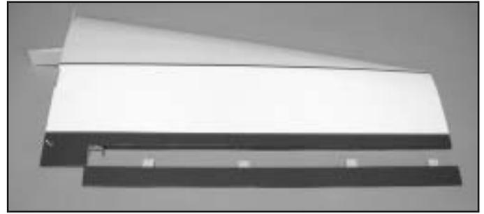
□ The ailerons are attached to each wing panel with four CA hinges. Slip the right aileron onto the right wing with the hinges in place. While holding the aileron in the proper position and flexing it downward, put a few drops of THIN CA on the top side of the hinge. Repeat for the bottom side. After the CA has "fired," check that the aileron is secure by giving it a firm tug.
