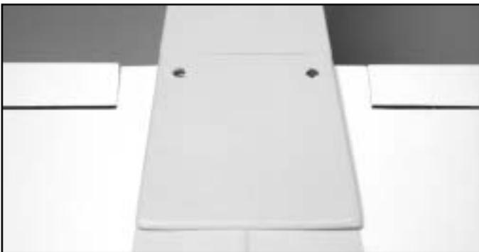
▢ Mount the wing to the fuse and install the rear wing fairing with CA.
