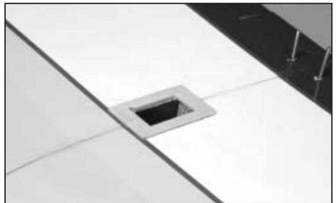
□ Locate the servo tray for the aileron servo. Put into place on the top of the wing and draw a line around the tray on the outside. Next draw a line around the inside of the servo tray. Set the servo tray aside and using a sharp modeling knife, cut along the inside line to remove covering and balsa sheeting for the servo to sit in. Now, using a sharp blade, lightly score along the outside line to remove the covering.
