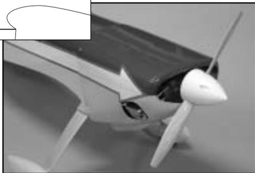
▢ With the engine in place, set the cowl onto the fuselage and mark the places on the cowl for the engine cylinder head and exhaust to exit the cowl. Remove the cowl and using a Dremel tool, cut away the areas previously marked on the cowl. Also, cut away to clear the prop shaft.
