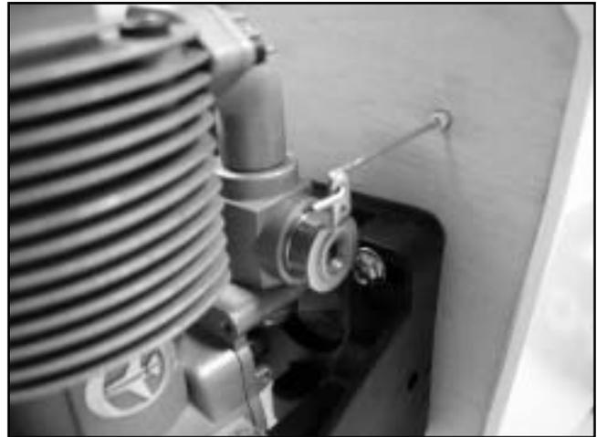
□ Install the throttle pushrod. You might need to screw off the throttle lever first then attach to Z-bend throttle pushrod end.
