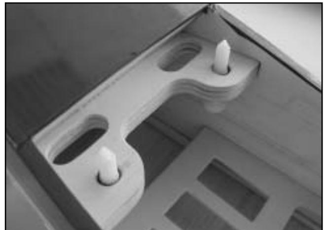
□ Screw the Wing Bolts inversely so the sharp ends just a little higher than the saddle of fuselage.
