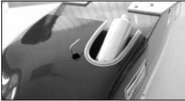
☐ Since the needle valve was not long enough to extend outside the cowl, we had to install an extension. Depending on the engine you use this may be necessary. We made ours out of the excess wire from the Aileron pushrod.
