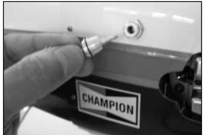
□ Before permanently installing the cowl, we have opted to install a Thunder Tiger #1115 Precision Fueler Valve. Set the cowl in place. Mark the holes for the cowl attachment screws and drill using a 1/16" drill bit. Attach the cowl using the four 2.6x8mm Wood Screws.
