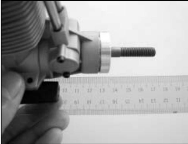
□ Locate the motor mount hardware: two beams, backplate, two anti-vibration rubber and four machine screws. Install the adjustable engine mount. Remember to install anti-vibration rubber to reduce the engine vibration. Set the engine on engine mount as shown, measure from the firewall to the front of thrust washer at 13.5cm(5 5/16"). Mark the engine mounting hole position on the engine mounts.
