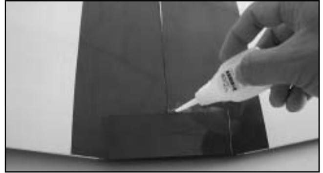
□ Apply a liberal amount of medium CA to the exposed wing panel and place the Wing Protector on it, holding it until the CA sets.
