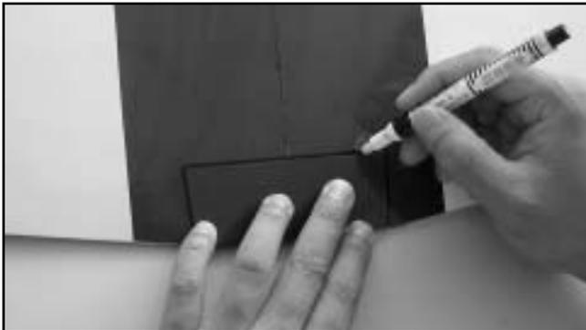
□ Measure the top and bottom to find center of the Wing Protector. This will be used to center the protector on the trailing edge of the wing panel. Place the protector on the wing panel and mark around the three sides with a pen or marker.
