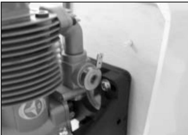
□ Drill a 3mm(1/8") hole for throttle pushrod guide tube. Install the pushrod tube and use a couple of drops of medium CA to hold in place in the firewall.
