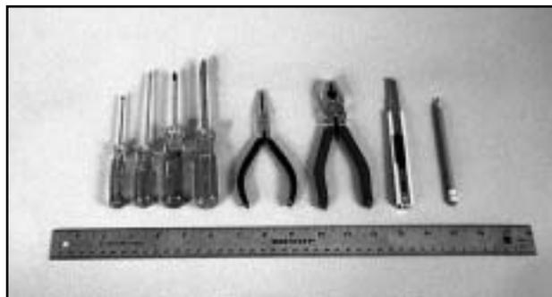
**Tools** - Model assembly can be much easier if the proper tools are used. Therefore, we have included in our checklist to the left, a complete listing of all the tools we used to assemble our prototype models. As you will notice, many household tools can be utilized during construction.
