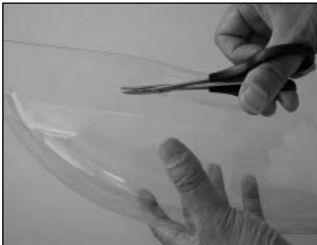
☐ Trim the canopy by using a pair of lexan scissors.
