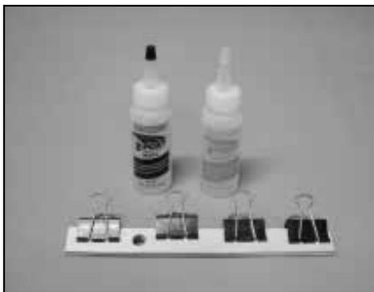
□ Next, use epoxy to laminate the two dihedral braces together, keeping the holes lined up. Clamp together as the glue sets. Wipe off excess glue with a paper towel wetted with rubbing alcohol.
