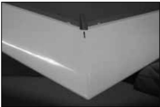
After the glue has set, test fit the right wing panel. Make sure the cables thread properly into the right wing. When satisfied, apply epoxy to the dihedral brace and the fuselage and join the right wing panel in place. Of course, you have to thread the cables through the root rib. Once again, make sure the slot for the power pod remains clear of glue.
