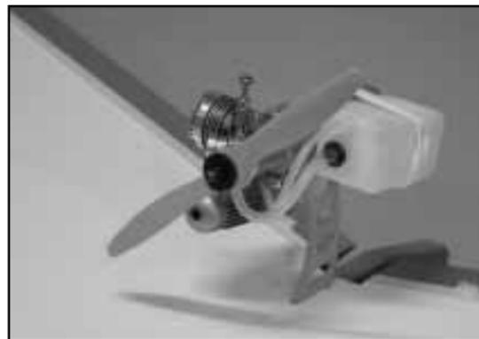
If you use the optional engine pod, mount the engine on the right side of the pod with the furnished hardware. Plumb the tank and mount it with a rubber band on the left side of the pod.
