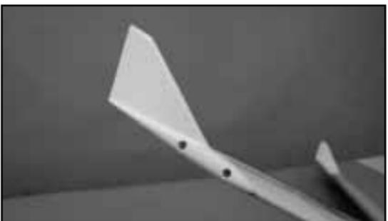
The two wing tiplets are attached with two screws. You will have to drill holes for the screws in both the tiplets and the wing tips.
