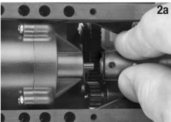
**2a** Disconnect the rear drive shaft from the transmission output shaft by removing the 4x7.5 yoke pin. Slide the drive shaft back toward the rear and leave the shaft attached to the rear differential.
