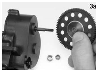
**3a** Disassemble the spur gear and slipper assembly by removing the 4.0NL and slide the whole assembly off of the shaft.
