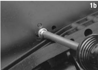
**1b** Remove the 3x10WM screw from the bottom of the carb linkage bell crank post. (Models equipped with TRX 2.5 Racing Engine only).
