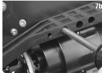
Set transmission back into the chassis and secure it with the eight 3x12RM screws.
