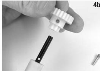
**4b** Remove the reverse primary gear (Part #4995) from the 2-speed primary shaft by removing the primary gear pin and set aside until step #5.
