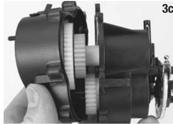
**3c** Gently separate the two transmission halves.
