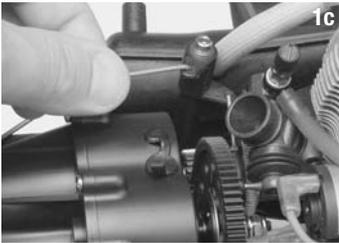
**1c** Lift the bell crank assembly off of the chassis (this is to provide access to the transmission).
