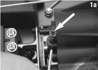
**1a** Begin by removing the air filter. Disconnect the shift linkage from the shift fork that exits the front of the transmission. Loosen the 3x3GS on top of the brake cam and remove the brake lever from the brake cam.
