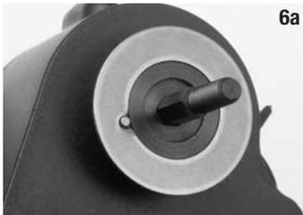
**6a** Place a slipper plate (#4625) over the slipper shaft followed by a pressure ring (#4622) and the metal spur gear bushing (#1994). Replace the slipper pegs if there is sign of wear or friction on either face of the gear. Note: The notch in the
