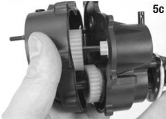
**5c** Connect the two transmission halves making sure that all gears and shafts are aligned correctly. Secure the transmission halves with the seven 3x10RST screws.
