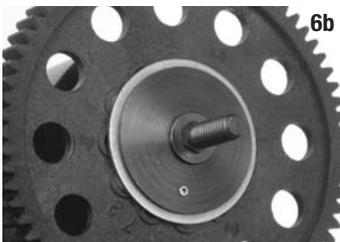
**6b** Fit the spur gear over the bushing followed by the second pressure ring and pressure plate.
