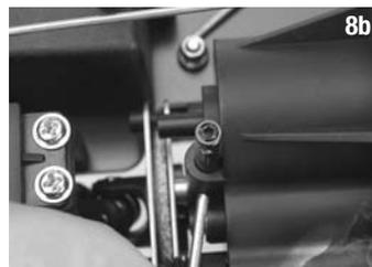
Insert the brake lever into the brake cam and tighten the 3x3GS. Connect the shift linkage back onto the shift fork by popping the rod end onto the ball stud. Install the air filter back onto the carburetor. This completes the single speed installation.
