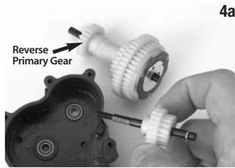
**4a** Remove the 2-speed primary gear shaft assembly and the 2-speed slipper shaft (#4992) from the transmission half.
