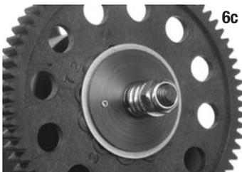
**6c** Slide the slipper spring (#1994) over the slipper shaft and secure the assembly with the 4.0NL. Tighten the slipper nut until it stops then back it off 1/4 turn.
