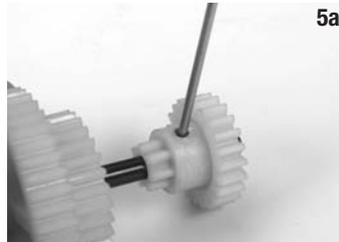
**5a** Locate the single speed primary shaft assembly. Remove the 5.0 E-clip from the primary shaft #5193. **Caution: Always wear eye protection when removing or installing E-clips to prevent injury.** Slide the reverse primary gear onto the single speed primary shaft
