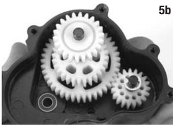
**5b** Place the complete single speed gear hub assembly into the transmission case half next to the new slipper shaft. Apply a light coating of grease to the gears (such as Traxxas lithium grease part #5148).
