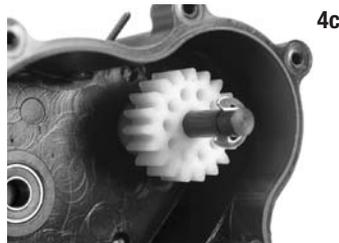
**4c** Locate the single speed slipper shaft (#5193) and insert the shaft into the transmission case half where the 2-speed slipper shaft was located.
