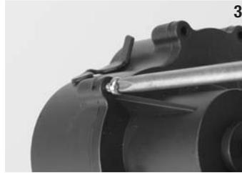
**3b** Remove the seven 3x10RST screws from the transmission case.
