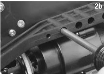
**2b** Remove the eight 3x12RM screws located in the chassis braces that secure the transmission to the chassis.
