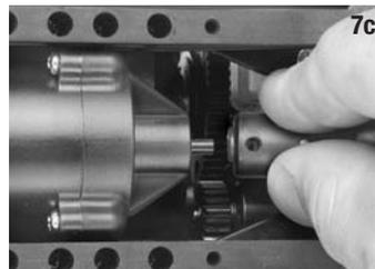
Reconnect the rear drive shaft to the output shaft of the transmission with the 4x5 yoke pin.
