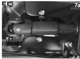
Place the front of the transmission down into the chassis first then key the short male drive shaft from the front differential into the short female drive shaft from the transmission.
