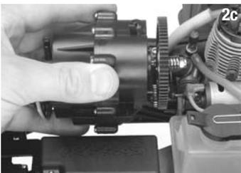
**2c** Lift the transmission from the chassis.
