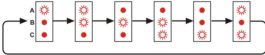
LED A-> LEDA,B -> LEDB -> LEDB,C -> LEDC -> LEDC,A -> this sequence will be repeated if the hall effect sensors are functioned properly.
