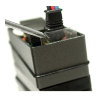
Install the lower servo case with 4 long screws, do not tighten. You will need to slide all 3 O rings into place before you tighten and secure the case.
