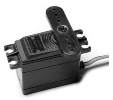
Remove the servo arm and be careful to keep the servo arm output shaft centered. Remove the 4 long screws located at the bottom of the servo. Notice that the long servo case screws have very small o rings on them.
