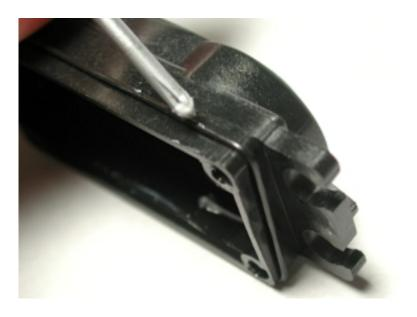
Install the upper case to the upper mid case. Do not slide the O ring into place as of yet.
