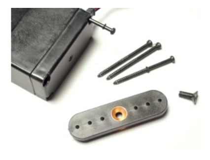
Using your two index fingers and your thumb, push down on the servo output shaft. After you have removed the top case, note the location of the output shaft pin. The pin should be in the straight or forward direction.
