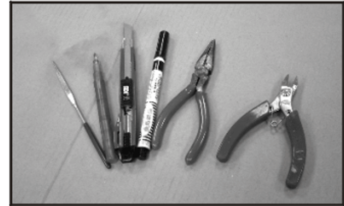
Tools for assembling: pliers · pincer pliers · screw driver, tweezers, a marker, a file, a cutter knife, quick-dry glue, clear tapes, fiber tapes, etc.
