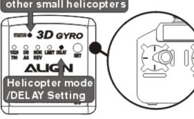
Move the transmitter rudder stick to the needed delay
