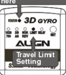
Move the rudder stick on your transmitter left until the tail pitch slider reaches the end. Repeat on the right until the tail pitch slider reaches the other end. Then press the "SET" button.
