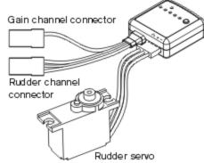
Gain and Rudder channel mapping diagram
