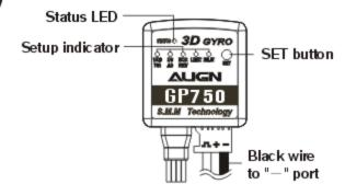
Connects to gyrogain channel on receiver (CH5/AUX) Connects to rudder channel on receiver (CH4/RUDD)
