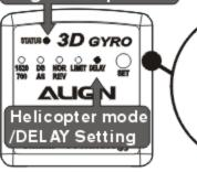
When paired with a T-REX 500/600/700, please remember to set the STATUS LED set the STATUS LED to green. If you want to set delay at the same time, please move the transmitter rudder stick to the direction where STATUS LED is green. With the DELAY STATUS LED flashing, the delay amount is adjusted by stick position from the center: percentage is 0% at middle stick position, and 100% at the end position.
