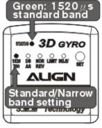
The GP750 is set to 1520  $\mu$  s at the factory. Use the rudder stick on your transmitter to select, and set it to green STATUS LED.
