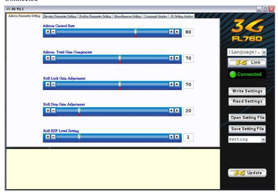
You can click "Write Settings" button to send the value to 3G. Or click "Read Settings" button to read current settings from 3G. The status will be show as linking up during writing or reading.
