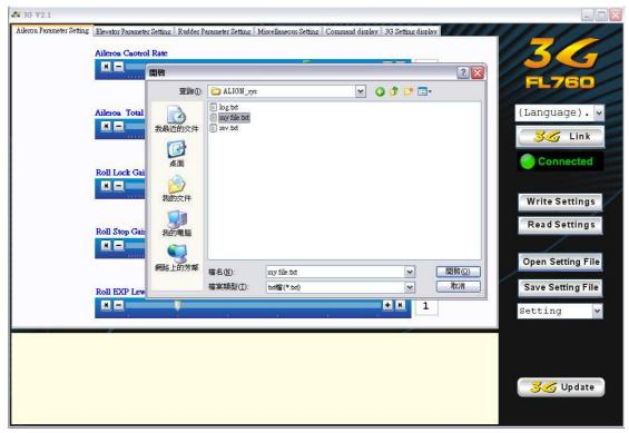
You can find the common settings in the dropdown list. There are 2 build-in setting as T-REX500~T-REX700 and T-REX250~T-REX450. Any saved setting will be appear in the list as well.
