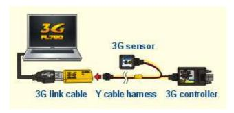
After turn on the 3G, click 3G link button to start connect PC and 3G controller unit. Below the "3G link" button you will see the connect status. The software will load the value in 3G controller automatically.
