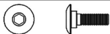
Socket button head collar screw 半圓頭內六角軸套螺絲(M3x8mm) x 8
