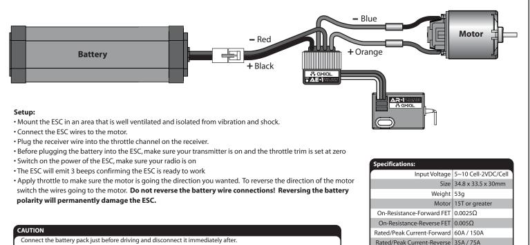
Always make sure you are connecting the ESC to a proper power source that has the correct voltage & polarity. Incorrect voltages or reversed polarity will damage the ESC.
