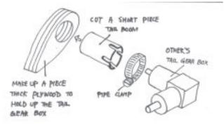
Century tail gearbox). Bond both wooden circles to each other and then bond below the F9 former using epoxy. Mark the centerline of the tail gearbox input shaft (simple when only one half of the gearbox is mounted to F10) and drill straight through with a drill bit that is 1/16" larger than the brass tubing.
