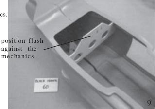
former and insert the brass housing through one of the large side holes. Position the F4 former behind the mechanics and initially position flush against the mechanics. While viewing from above, mark on the brass housing the position that will be approximately 1/2" past the end of the tail coupling. Trim the brass housing at the marked location and remove the mechanics and reposition the brass housing now inserted into the center hole in the F4 former.
