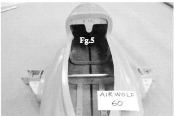
5. Cut the clear windshield to fit inside of the front nose, useing "GOOP "or "Zap A-Dap-A Goo" silicon base type glue to attached to front nose. Note! Do not over cut the plastic.See Fg.6
