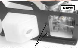
IMPORTANT: Motor mount screws DO NOT have thread lock yet. Loosen these screws to position the motor or replace with optional #HW3018A for .50 size engines.
