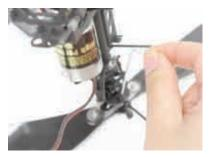
If the helicopter does not seem to turn properly or the tail motor seems to make a gritty sound as it tries to turn, check the gear mesh. If the gear mesh is too tight, this will cause excessive wear on the tail motor shortening it's life and degrading performance. If the gear mesh is too loose, the tail will simply not respond well enough. Adjust the two screws that hold the motor in place in order to realign the mesh.
