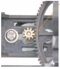
If the helicopter does not seem to have enough power or the motor sounds like the motor is being bogged down, check the gear mesh. If the gear mesh is too tight, it can cause unnecessary wear to the main motor. If too tight, the gear mesh will shorten the life of the main motor and degrade performance in the model overall. To adjust the gear mesh, loosen the two screws holding the motor in place and realign.
