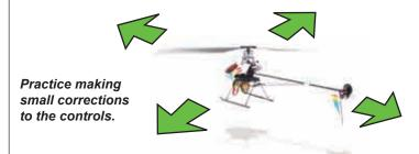
Only slight inputs are needed to move the helicopter. Too much input can cause the helicopter to tip too far to one side. Continue to make small corrections to keep it level.
