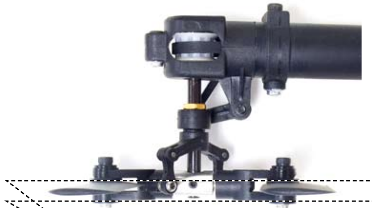
Tail rotor blades with zero pitch (blade tips will be in-line)
