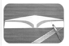
NOTE: Be very careful not to cut or score the balsa underneath as this might cause structural failure in flight.
