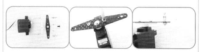
• If you use mini serv, install the long servo arm(dual, high performance, made of carbon fiber) onto the servo of rudder.
