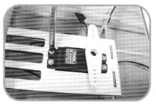
• Insert the control horn(dual) into the slot and fix it with glue.
