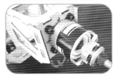
• Use the supplied bolts and washers to mount the motor to the mounting plate. put a drop of thread lock on the mounting bolts.
