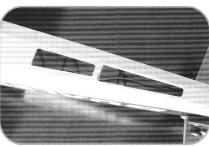
• Remove the covering from the bottom of the fuselage as it is shown in order to allow cool air to escape from the fuselage.
