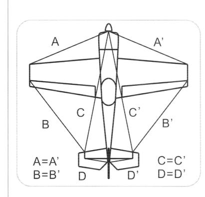
Adjust the aircraft and make sure both of the sides are symmetric, like the diagram . So that the plane is ready for flight.
