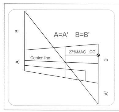
Measure the CG from the leading edge of wing root rib, Adjust the battery pack location. For CG proper position should be at 25-30%MAC. This recommendation balance point is for your first flights. The CG can be moved around later to fit your personal taste.
