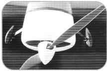
Note: Do not use the damaged or cracked propeller and spinner, which can be broken at high speed and can cause serious damage to body and property!
