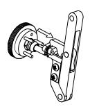
Pull the handle away from the flywheel. The clutch shoe and spring will slide away from the flywheel.
