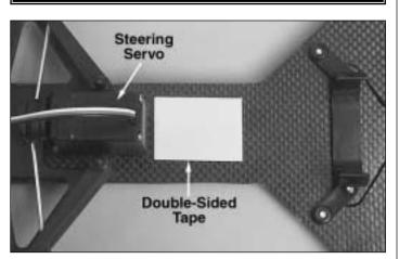
□ 1. Install a large piece of double-sided tape onto the chassis directly behind the steering servo. Install the receiver onto the double-sided tape. Install the receiver in the direction shown in the following step. Note: Do not worry about the receivers antenna wire at this point. It will be installed once the battery has been installed.
