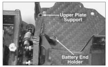
$\Box$  2. Install (1) of the battery end holders (21) directly in front of the upper plate support (8).
