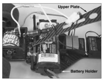
□ 4. Re-install the upper plate onto the chassis of the Delphi Indy car. Secure the front of the upper plate to the chassis using the previously removed body clips. Note: If you completely removed the upper plate from the chassis you must re-install the rear shock.
