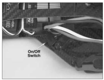
□ 2. Secure the ESC's on/off switch to the chassis using a small piece of double-sided tape. Make sure that you place the switch in a position where it will not get turned "off" during running.
