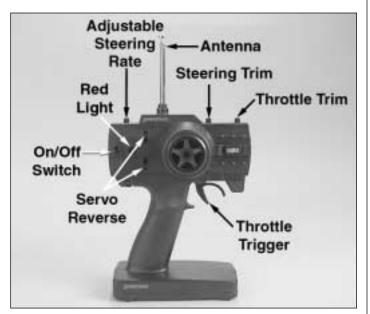
□ 3. Install the transmitter antenna by screwing it into the hole on the top of the transmitter. Give the antenna a quick tug to make sure it is securely attached.
