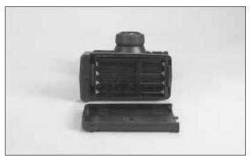
□ 4. Slide open the battery door on the bottom of the transmitter. Install eight (8) "AA" batteries into the transmitter in the configuration molded into the plastic on the battery holder. Re-install the battery door.
