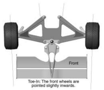
Toe-in and toe-out refers to the angle at which the tires point when viewed from above. Toe-in increases stability under acceleration and helps straight away tracking. Toe-out will increase steering going into corners, but will decrease the overall stability during acceleration. The front typically is set-up with 0 to -2 degrees of toe-in. Only use a toe-out setting when you are running on a short track with many turns and few straights.
