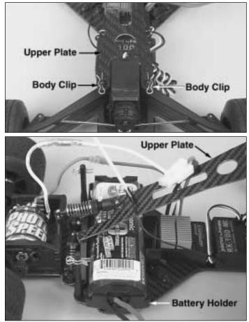
□ 7. Remove the body clips from the upper plate posts and lift the upper plate away from the chassis. Install the charged 6 cell battery into the battery slot. Re-install the upper plate onto the Delphi Indy car as shown above. Re-install the body clips into the upper plate posts.
