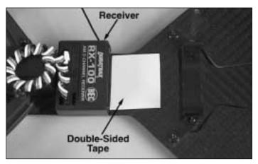
□ 1. Install a large piece of double-sided tape on the chassis directly behind the receiver for the ESC to mount to. Mount the ESC onto the double sided tape. Connect the motor wires to the motor (white to white, blue to blue).
