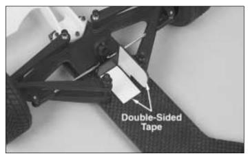
□ 3. Install a piece of included double-sided tape to the inside of the servo mount and a piece to the chassis as shown.
