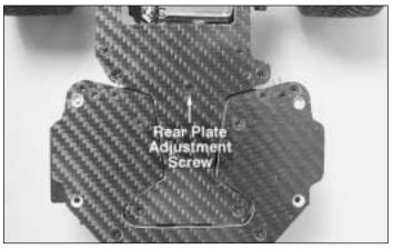
The side to side stiffness of the rear plate is easily adjustable by tightening or loosening the center pivot. A stiff setting will give you a more consistant feel but slightly less rear grip (the wheels may spin out easier but it won't break-loose as suddenly). A softer setting will increase initial rear grip but may tend to break loose more suddenly. Typically a tighter setting is more predictable at high speeds and softer setting more predictable at lower speeds.
