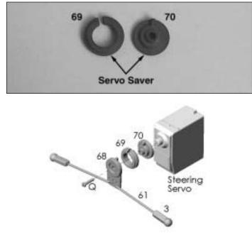
□ 5. Locate the two servo saver parts (69) and (70 FUT, AIR, HTEC, or MUL, depending on your servo brand) and install them onto the pre-mounted servo saver part (68). Install this
