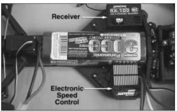
□ 3. Remove the ESC and receiver from behind the steering servo and install them onto the sides of the main chassis using double sided tape.
