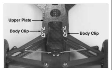
□ 1. Remove the upper plate by removing the two body clips in the front and lifting the front of the upper plate up out of the way. Note: To completely remove the upper plate you must first detach the rear shock from the upper plate.
