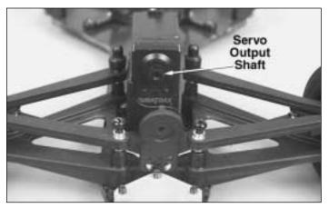
□ 4. Install the servo onto the chassis, securing it in place with the double-sided tape. Note: The servo needs to be mounted so that the output shaft is in the upper position as shown.
