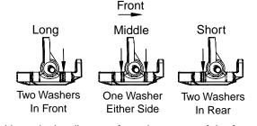
Wheel base is the distance from the center of the front wheel to the center of the rear wheel. Lengthening the wheel base of the Evader increases steering, but decreases rear traction as a result of increased weight distribution to the front wheels. Decreasing the wheel base of the Evader will increase rear traction, but decrease steering.
