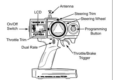
$\Box$  4. Install the transmitter antenna by screwing it into the hole on the top of the transmitter. Give a light tug on the antenna to be sure it is seated properly.
