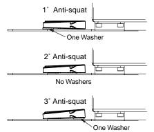
Increasing rear anti-squat will increase traction and give you more on-power stability. However, the buggy will have less grip when decelerating into a corner. This could cause the buggy to spin out entering the corner. More anti-squat allows the buggy to accelerate better through the rough parts of the track.
