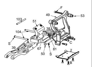
9. Attach the front bumper (2) to the front bulkhead using four 4-40x5/16" (B) flat head machine screws.
