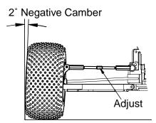
Camber refers to the angle at which the tire and wheel ride in relation to the ground when viewed from the front or rear. Negative camber is when the tire and wheel lean inward and positive camber is when the tire and wheel lean outward. Typically you want 0 to 2 degrees of negative camber. Never put in positive camber. Make sure that both sides have equal amounts of camber by keeping the camber turnbuckles equal in length.
