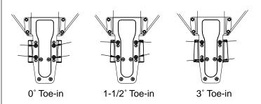
Rear toe-in affects the traction of both the front and rear of the buggy. Rear toe-in increases the amount of traction in the rear, but decreases steering. Decreasing rear toe-in will increase steering, but will give less rear traction. Notice that placing the rear suspension arm mount screws in different locations on the aluminum rear plate changes the rear toe-in.
