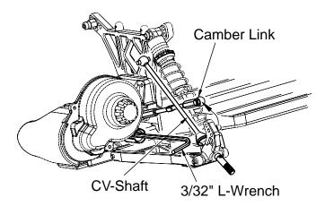
While holding the left rear tire, tighten the adjusting screw by inserting the included 3/32" L-wrench into the cap screw on the right side of the ball differential. The screw should be tightened until it is "just snug." **Caution: Do not over tighten the adjusting screw or you will damage the differential.** Next, loosen the screw 1/8 of a turn.
