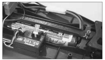
□ 8. Install the charged 6 or 7 cell battery into the battery slot (remove foam if using a 7-cell). Re-install the battery strap onto the Evader BX Pro. Note that there is a channel in the chassis for the battery strap to rest in. Re-install the body clip into the battery strap post.
