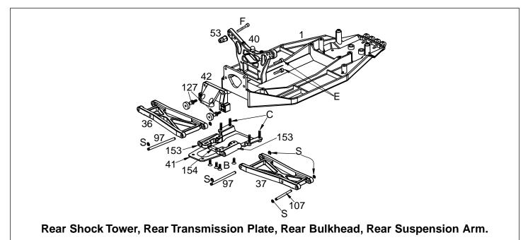
1. Attach the rear chassis plate (41) to the chassis using four 4-40x3/8" (C) socket head screws.
