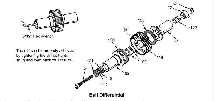
**1.** Place one of the differential thrust washers (121) onto the 3x25mm cap screw (G).
