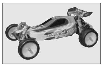
□ 9. Decal the body as desired and install on the chassis, using two body clips to secure in place.
