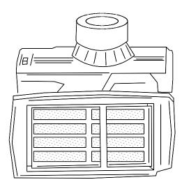
□ 5. Slide open the battery door on the bottom of the transmitter. Install eight (8) "AA" batteries into the transmitter in the configuration molded into the plastic on the battery holder. Re-install the battery door.
