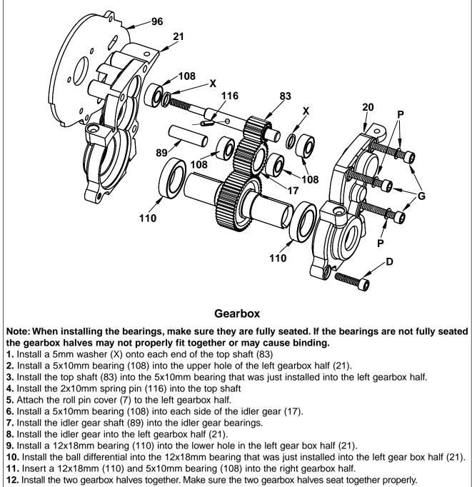
13. Secure the two halves together with the 4-40x1/2" socket head screw (D).
