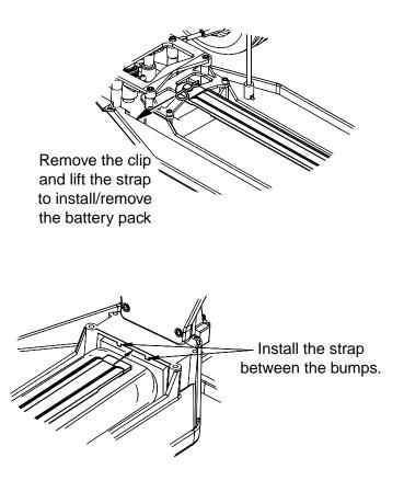
□ 7. Remove the body pin from the battery strap post and remove the battery strap from the Evader BX Pro.
