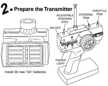
Screw in the transmitter antenna and install the "AA" batteries. Check to make sure the red power light glows when turning the switch "on".
