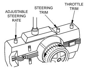
To make your Evader drive in a straight line, you may need to adjust the steering trim knob located on the transmitter. Adjust the dual rate knob to increase or decrease the steering travel. When first learning to drive, adjust the dual rate knob for less steering travel. As you get to be a better driver, adjust the dual rate knob for more steering travel.
