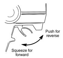
Hold up the rear wheels and squeeze the trigger. The rear wheels should spin forward. Push the trigger back. The rear wheels should spin backwards. If the wheels spin with the trigger in the neutral position, adjust the throttle trim knob located on the transmitter.
