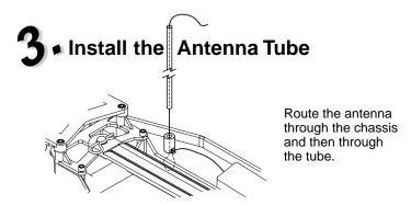
Install the antenna to the chassis. Secure excess wire to the tube using tape. **DO NOT CUT THE ANTENNA WIRE!!!**
