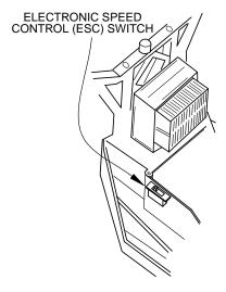
Turn on the switch in the chassis located on the right side of the chassis.
