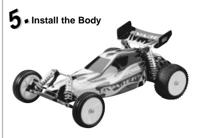
Place the body onto the chassis. Use clips to secure the body in place. Install the wing into the rear shock tower.
