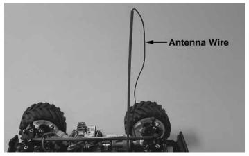
□ 5. Straighten the receiver antenna. Run the receiver antenna wire through the included antenna tube. DO NOT CUT OR COIL THE ANTENNA WIRE. Press fit the antenna tube into the antenna mount hole. **TIP:** Run the antenna wire through your finger to straighten out the kinks before running through the antenna tube. Also applying a small amount of soap and water to the antenna wire will help lubricate the wire for threading into the antenna tube.
