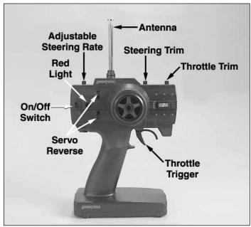
☐ 2. Install the transmitter antenna by screwing it into the hole on the top of the transmitter. Give the top of the antenna a light tug to make sure that it is properly secured to the transmitter.
