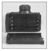
☐ 4. Turn on the transmitter using the on/off switch (see step #3). The red light on the transmitter should light up. If there is no light on, turn the transmitter off and check to ensure that the batteries are making contact with the metal contacts in the battery holder. Make sure the batteries are installed correctly. Turn the transmitter on and check for the red light. If the red light appears, turn off the transmitter. If the red light blinks, the batteries are low and should be replaced.
