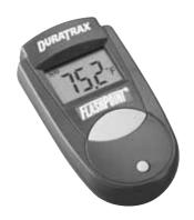
The DuraTrax® FlashPoint™ Temperature Gauge is a non-contact infrared thermometer. Specifically designed for use with R/C engines, batteries, motors, sealing irons and heat guns, simply aim the temperature gauge at the target and press the measurement button to quickly and easily display the surface temperature! The distance to target ratio is 1:1, and therefore the temperature gauge should be positioned as close to the target as possible.
