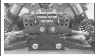
**Step 5.** Gently spread the gearbox halves apart enough for the stabilizer bar to fit into the molded stabilizer bar holders.
