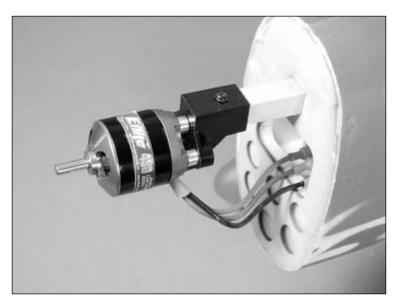
5. Check the operation of the motor using the radio system. The motor should rotate counterclockwise when viewed from the front. Follow the instructions included with the speed control if necessary to reverse the direction of rotation of the motor. Secure the speed control inside the fuselage using hook and loop tape.
