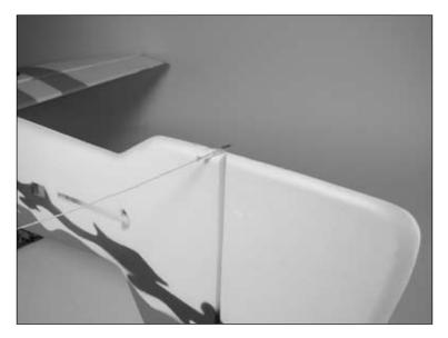
O 6. Wrap a small piece of tape on the string where it crosses the wing tip. Mark the tape to indicate the exact location of the wing tip. Swing the tape over check the position of the opposite wing tip. If these are not equal, reposition the wing and tape and repeat until the mark on the tape aligns with both wing tips.
