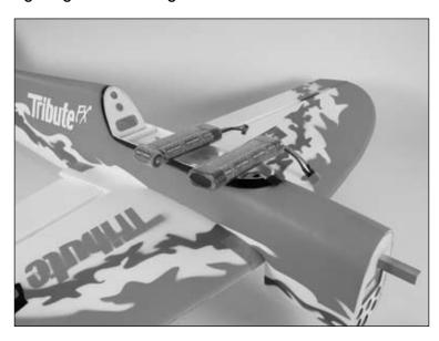
11. Use thick foam-safe CA to glue the belly pan to the wing. It may be necessary to lightly sand the belly pan to fit perfectly to the contour of the wing.
