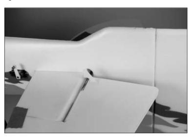
7. Slide the control horn backplate down on the control horn from the top side of the elevator. The backplate rests tight against the elevator. Use foam-safe CA on the backplate to complete the control horn installation.
