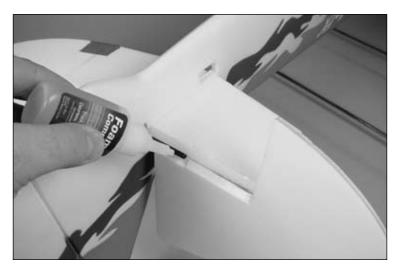
**Hint**: Use low-tack tape to hold the two elevator halves in neutral while the CA fully cures to ensure they are in alignment with each other.
