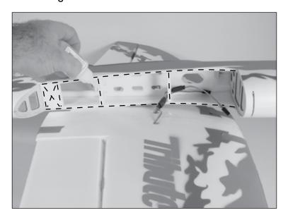
O 10. Place a support under the wing so the fuselage is not touching the work surface. Use weights to hold the fuselage tight against the wing while the CA cures.
