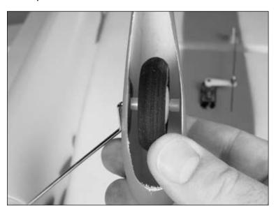
6. Position the wheel pant so it is not touching the work surface when the plane is resting on the tail skid and wheels.
