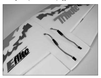
3. Rest the fuselage on the wing. Guide the servo extensions above the former as shown.
