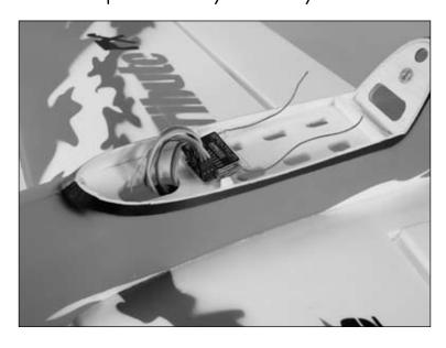
**Note**: Never cut the receiver antenna as this will greatly reduce the range of your radio system.
