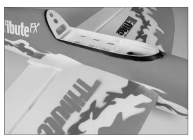
8. Check the alignment of the wing to the vertical stabilizer to make sure the wing is perpendicular to the wing. Lightly sand the fuselage wing saddle if there is an alignment correction to be made.
