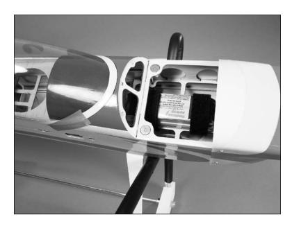
**Note**: Place a piece of hook and loop tape on the bottom of the battery and on the fuselage where the battery rests. This will keep the battery from shifting forward or backward during extreme maneuvers.
