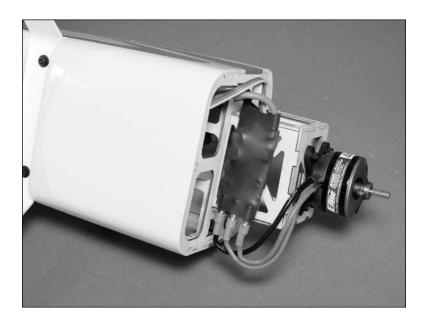
2. Connect the speed control to the radio system and motor battery. Check that the motor is rotating in the correct direction. It will rotate counterclockwise when viewed from the front of the aircraft. Use the instructions with your speed control to correct a motor that is operating in the wrong direction.  3. Slide the propeller adapter through the hole in the propeller.
