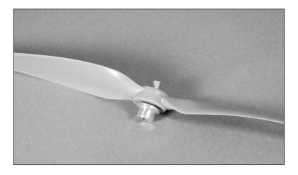
4. Slide the <sup>1</sup>/<sub>2</sub>-inch (13mm) plastic washer onto the adapter.
