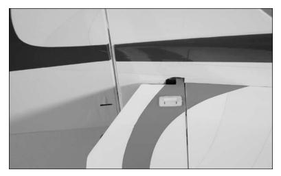
4. Install the micro control connector onto the elevator servo arm. Pass the elevator pushrod wire through the connector. With the radio on and elevator trim centered, center the elevator. Secure the elevator pushrod wire using the 2mm x 4mm screw and a small Phillips screwdriver.
