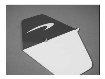
2. Remove the covering from the blind nuts in the wing using a hobby knife. Attach the Side Force Generator to the wing.
