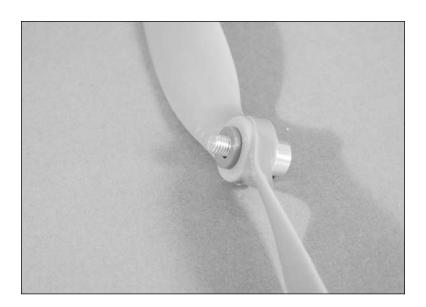
5. Slide the spinner backplate onto the adapter. Thread the propeller nut onto the adapter, but do not tighten it at this time.
