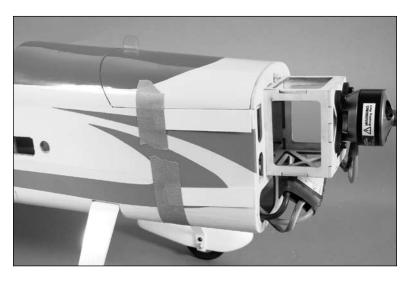
7. Slide the cowling on the fuselage. With the propeller adapter on the motor shaft, position the cowl so there is a gap between the spinner and cowling.
