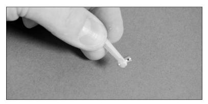
8. Turn on the radio system and center the aileron trim and stick. Make sure the aileron servo is operating properly using the transmitter. Slide the pushrod wire through the micro connector. Install the servo arm parallel to the aileron hinge line. Center the aileron, and secure the position of the wire using the 2mm x 4mm screw and a Phillips screwdriver.
