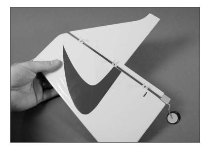
3. Place the fin in position on the fuselage. Trace the outline of the fuselage onto both sides of the fin.
