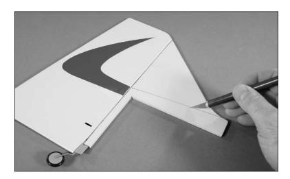
5. Position the fin back onto the fuselage. Use a square to check the alignment between the fin and stabilizer. Lightly sand the bottom of the fin until the alignment is correct.
