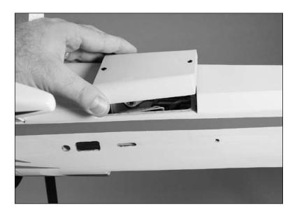
3. Place the canopy into position on the fuselage. Use a felt-tipped pen to trace the outline of the canopy onto the fuselage.
