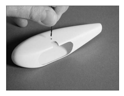
O O 6. Secure the pant to the landing gear with a 2mm x 6mm wood screw.
