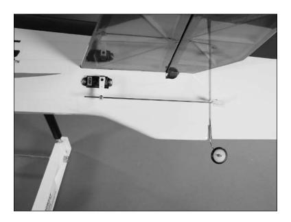
6. Attach the 8-inch (204mm) carbon stabilizer supports between the fuselage and stabilizer. Make notches in the stabilizer and fuselage for the rods to rest in. Secure the rods using 6-minute epoxy.
