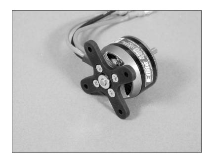
Attach the Outrunner motor to the front of the firewall using four black #4 washers and four 4-40 x <sup>3</sup>/<sub>8</sub>-inch socket head screws.
