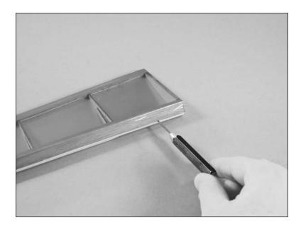
2. Slide four hinges into the slits in the aileron. Center the slot in the hinge with the hole drilled in Step 1. Place a T-pin in each hinge to prevent it from being pushed into the wing when installing the aileron.
