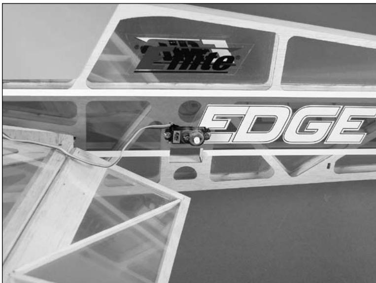
**Note:** Notch the fuselage so you can pass the elevator servo lead to the same side of the fuselage as the aileron servo leads.
