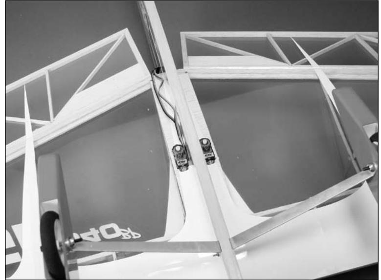
**Hint:** Pass both servo leads to the same side of the fuselage for a cleaner radio installation.
