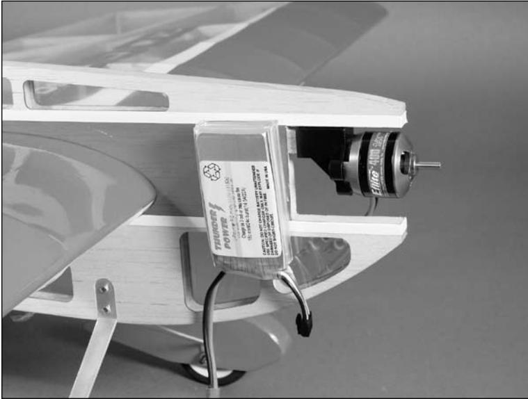
**Note:** Never check the motor rotation on the bench with the propeller installed. The plane could move and cause serious injury. Always check the motor without the propeller to avoid injury.
