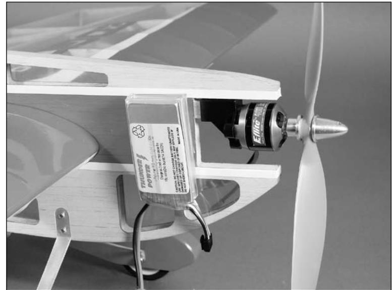
**Note:** The following image shows the installation of the Park 450 motor with correct spacers between the motor and mount.
