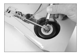
7. Place the retract on a flat surface. The mount for the retract and the axle will rest flat on the surface. Use a 2.5mm hex wrench to tighten the two screws on the axle enough to mark the axle. This will align the wheel so your model will taxi correctly when on the runway.
