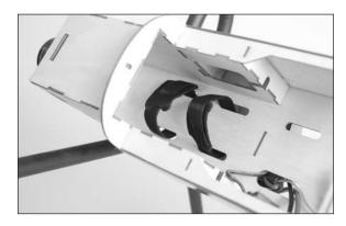
7. Place a piece of hook and loop tape on the battery floor, as well as on the bottom of the battery. This will keep the battery from sliding fore and aft in the fuselage.
