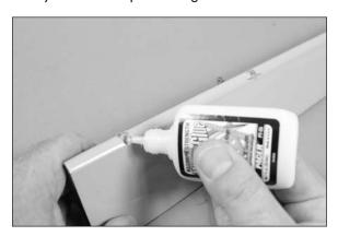
21. Apply hinge glue in the holes for the hinges in the trailing edge. Insert the flap hinges into the trailing edge of the wing. Repeat Step 16 and 17 to check the position of the hinges. Wrap a small amount of low-tack tape around the flap and inner trailing edge, and around the flap and aileron to keep it in position. Set the wing aside to allow the adhesive to fully cure.
