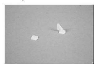
20 17. Use a #1 Phillips screwdriver and two 2mm x 8mm sheet metal screws to attach the control horn to the aileron.
