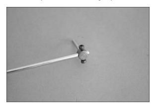
3. Slide the main wheel on the axle. Use a wheel collar and 1.5mm hex wrench to temporarily attach the wheel. Use a felt-tipped pen to mark the axle against the outer edge of the collar.
