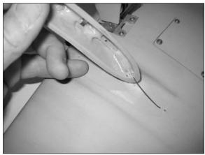
8. Use a #0 Phillips screwdriver to install a screw #1 x 1/4 wood screw into the skin. Remove and harden the hole with thin CA. Once complete install the pylon.
