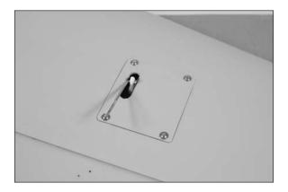
OO 16. Use a hobby knife with a #11 blade to remove the control horn backplate from the control horn. Discard the backplate as it will not be used when installing the control horn.
