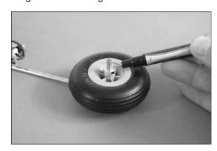
4. Remove the wheel collar and wheel from the axle. Use a rotary tool and cut-off wheel to trim the axle at the mark made in the previous step. Use a flat file to make a flat area on the first 1/4-inch (6mm) of the axle for the setscrew of the wheel collar to rest on when it is tightened.
