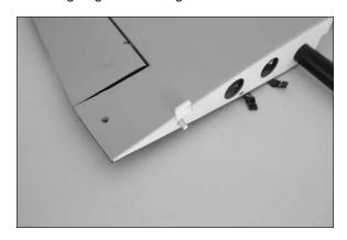
3. Slide the two wing panels together. They will fit tightly against each other as shown.
