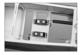
4. Plug a Y-harness into the aileron and flap port of your receiver. Plug the special Y-harness included with your E-flite retracts into the gear port of the receiver. Plug in a 3-inch extension into the Aux2 port if using the operational bombs or drop tanks.
