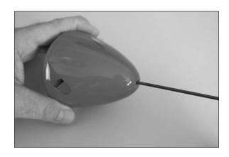
2. Check the rotation of the motor using the radio system. It must spin counterclockwise when viewed from the front of the fuselage. If not, reverse any two of the motor leads to correct the direction of rotation. 3. Slide the propeller adapter and spinner backplate (the included spinner does not have the lightening holes as shown in the photo) on the motor shaft. Leave a slight gap of 3/32-inch (2mm) between the backplate and cowling so the backplate does not rub on the cowling.
