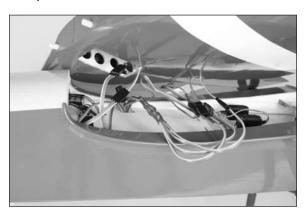
5. Place the wing on the fuselage. Make sure the leads are tucked in and not exposed between the wing and fuselage. Use two nylon wing bolts and a flat blade screwdriver to secure the wing to the fuselage.
