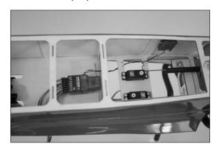
7. Use the hook and loop straps to secure the motor battery in the fuselage. Check that the power switch is set to the OFF position and connect the leads from the motor battery and speed control.
