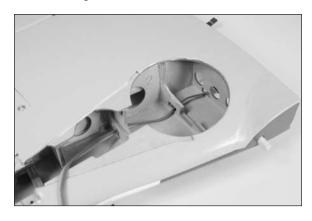
11. Use four 3mm x 8mm sheet metal screws to secure the retract in the wing. Check the operation of the retract using the radio system.
