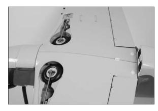
6. Slide the radiator scoop in position. The notch in the scoop fits the tab on the wing. The scoop is connected to the fuselage using a magnet.
