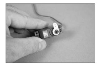
OO 6. Apply 2–3 drops of thin CA in each of the mounting holes for the servo screws. This will harden the wood and help prevent the screws from vibrating loose.
