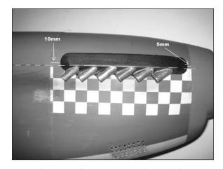
Gun history with the P-51 B and C model Mustang. Reference photos showing a few B and C models with (6) .50-caliber machine guns, three in each wing. Originally they were equiped with (4) .50-caliber guns. We have included a small plastic fairing with three gun barrels for you if you wish to use them. Your model comes with the simulated four (two per wing) .50-caliber guns. You may choose to remove the wooden guns that are installed and install the plastic guns if you choose.
