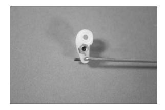
15. Slide the rudder pushrod into the tube in the fuselage. The pushrod from the tail wheel will slide into the brass pushrod connector. Secure the servo horn to the rudder servo using the screw removed in Step 1 and a #1 Phillips screwdriver.
