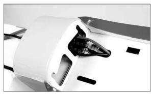
4. Connect the motor and speed control leads. If you are using the recommended motor and speed control, connect the lead wires according to color for the motor to rotate in the correct direction. Secure the leads so they do not interfere with the operation of the motor.
