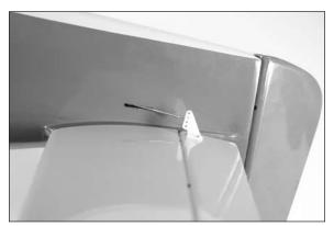
13. Attach the servo horn to the servo for the elevator servo using the screw removed in Step 1 and a #1 Phillips screwdriver. The elevator pushrod is connected to the hole enlarged in Step 9 using a nylon pushrod connector.
