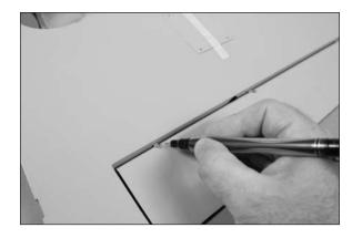
20. Remove the flap from the wing. Make sure the hinges are removed from the flap and wing at this time. Apply a small amount of hinge glue in each of the holes in the control surface for the hinges. Insert the hinges so the hinge point aligns with the mark made in the previous step. Allow the adhesive to fully cure before proceeding.
