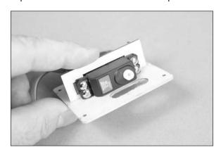
OO 6. Use the radio system to center the aileron servo. Place the servo horn on the servo so the longer portion of the arm is parallel to the servo center line. If the horn does not align, rotate the horn 180-degrees, as there are an odd number of splines on the servo output. Use a felt-tipped pen to mark the arm that protrudes through the servo cover.
