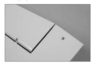
OO 18. Check that the flap can move through its range of motion. If there is binding, reposition the hinges and recheck the flap operation.
