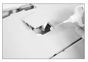
15. Use four 2mm x 8mm sheet metal screws with shoulder and a #1 Phillips screwdriver to secure the flap servo cover to the wing. You can remove the mark made earlier when the cover was removed using rubbing alcohol and a paper towel.
