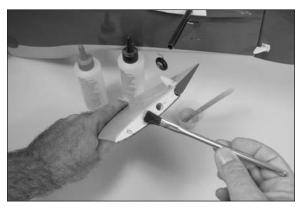
9. Slide the stabilizer back into position. Use rubbing alcohol and a paper towel to remove any epoxy that has oozed out before it has a chance to cure. Also check that the stabilizer tube is still positioned correctly in the fuselage.
