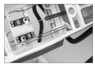
OO 16. Slide a clevis retainer on a nylon clevis. Thread the clevis on the elevator pushrod wire. When the connector is attached to the outside hole on the elevator control horn, the elevator should be centered with the elevator servo centered. Adjust the position of the clevis as necessary to align the elevator in the neutral position. Once set, slide the silicone retainer over the forks of the clevis so the clevis does not open accidentally in flight.
