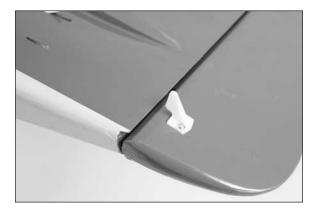
Attach the control horns to the elevators using 2mm x 8mm sheet metal screws and a #1 Phillips screwdriver.
