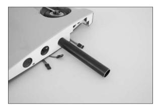
Insert the aluminum anti-rotation pin near the trailing edge of the wing.
