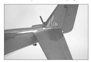
OO 8. Remove the stabilizer from the fuselage. Mix 1/2 ounce (15mL) of 12-minute epoxy. Apply the epoxy to the stabilizer tube, exposed wood on the fuselage, in the stabilizer tube socket of the stabilizer and to the exposed wood on the stabilizer root.
