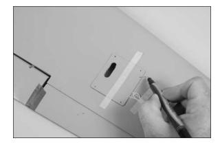
2. Remove the flap and aileron servo covers from the wing. Use a covering iron to seal the covering if the tape has lifted it from the wing or servo covers. Set the wing and flap servo cover aside.
