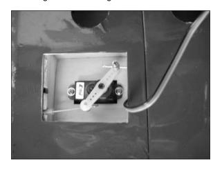
6. Insert the cable into the pushrod housing in the wing panel. You will find it will make an indentation in the bottom of the wing covering where it exits. Using a hobby knife and #11 blade, slice a small hole in the covering where the cable exits.
