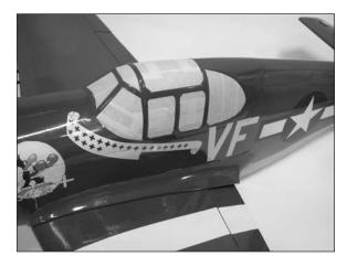
3. Use a heat gun and covering iron to ensure all sections of covering are ironed down and smooth with no wrinkles. Take your time here and make this right. Heat is the key, not pressure.
