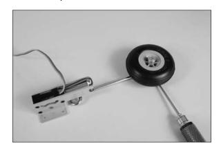
OO 8. Remove the axle from the main gear. Use a flat file to make flat areas on the main gear strut for the screws to rest. This will keep the axle from rotating if you encounter less than perfect landings.
