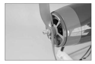
5. Fit the spinner cone in position. Make sure the openings for the propeller do not contact the propeller. Use a 3mm hex wrench to tighten the bolt that secures the spinner cone to the adapter.
