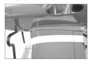
9. When balancing your model, support the plane inverted at the marks made on the top of the wing with your fingers or a commercially available balancing stand. This is the correct balance point for your model. Make sure your model is assembled and ready for flight before balancing.
