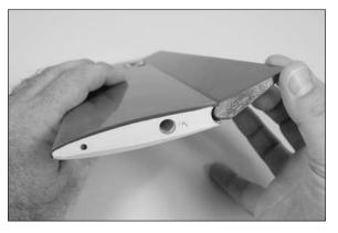
12. Remove the control surface and apply a small amount of hinge glue in each of the holes in the fixed surface for the hinges. Insert the hinges, attaching the control surface and fixed surface. Allow the adhesive to fully cure before proceeding.
