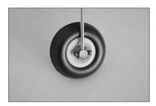
O 6. With the gear in the UP position, place it in the wing. Check that the wheel is centered in the opening when the mounting holes are aligned for the retract. Adjust the position of the wheel if necessary. Use a felt-tipped pen to mark the edge of the axle on the strut as shown.
