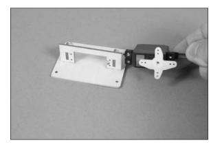
4. Remove the servo horn from the servo. Use side cutters to remove the arms from the horn that were not marked in the previous step. Enlarge the hole in the servo horn that is 7/16-inch (11mm) from the center of the horn using a pin vise and 5/64-inch drill bit.
