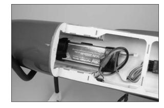
8. Center the rudder and elevator trims on the transmitter. Set the throttle stick to the low throttle position. Turn on the transmitter, then the receiver. Place the servo horns on the rudder and elevator servos as shown. Use a felt-tipped pen to mark the servo arms as shown in the photo. These will be the arms the pushrods will be connected to.
