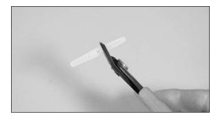
O 7. Use a pin drill and 5/64-inch (2mm) drill bit to enlarge the outer hole on the servo arm.
