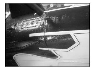
2. Once you are sure that you have cut through the hatch joints, use a small amount of force to rock the hatch in a rolling motion side to side. A small amount of movement should break any missed glue joints. Remove the hatch/fan assembly.
