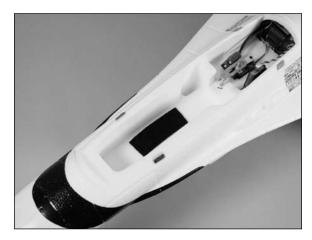
3. Place the battery into the battery compartment in the fuselage. The battery will be positioned as far back in the compartment as possible to achieve the correct Center of Gravity when you are using the recommended setup.
