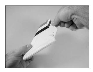
7. Check the fit of the stabilizer to the fuselage. Note that the control horn on the stabilizer will face toward the bottom of the fuselage when the stabilizer is installed.
