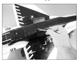
4. Insert the main landing gear into the slot in the bottom of the fuselage. You will need to flex the gear inward slightly to get it to fit into the slot.
