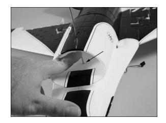
19. The nose gear will slide into the hole in the steering arm as its final destination. The screw at the steering arm will then be tightened so it is resting in the flat area made in Step 16. Use a #1 Phillips screwdriver to tighten the screw in the steering arm. Always remember to use threadlock on metal-to-metal fasteners to prevent them from vibrating loose.
