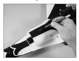
O 17. Slide the nose gear into the slot from the bottom of the fuselage. You will need to slide the gear wire through the 1/16-inch wheel collar before it continues its journey into the fuselage as shown in the following photos.
