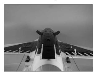
3. Use a hobby knife with a #11 blade to remove the decal from the bottom of the fuselage to expose the slot for the main landing gear.
