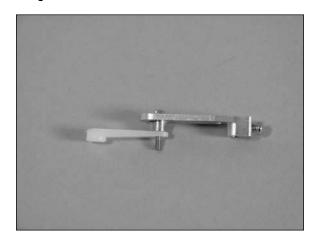
11. Thread a 2mm nut onto the screw from underneath the servo arm. Tighten the screw and nut to secure the bushing and steering arm. Always use threadlock on metal-to-metal fasteners to prevent them from vibrating loose.
