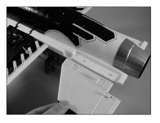
O 8. Use two 2mm x 12mm self-tapping screws and a #1 Phillips screwdriver to secure the stabilizer to the fuselage. Use care not to over-tighten the screws and cause damage to the fuselage or stabilizer.
