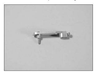
10. Use a #1 Phillips screwdriver to start the screw into the outermost hole in the servo arm. Tighten the screw so the brass steering arm bushing is tight against the servo arm.
