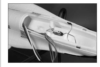
D 14. Locate the nose gear. Notice there is a slight bend to the gear wire. This bend will angle the gear forward in a scale-like manner when it has been installed.
