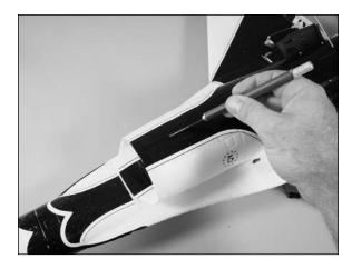
O 18. Slide the nose gear into the slot from the bottom of the fuselage. You will need to slide the gear wire through the 1/16-inch wheel collar before it continues its journey into the fuselage as shown in the following photos.
