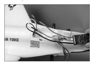
2. Apply a small piece of hook and loop tape to the bottom of the speed control.
