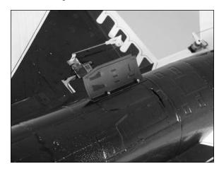
Repeat Step 1 to install the remaining gear door on the bottom of the fuselage.
