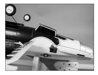
Repeat Steps 1 and 2 to install the remaining ventral fin on the bottom of the fuselage.
