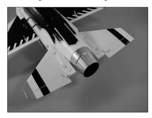
**Note**: The stabilizer tips will be lower than the center of the stabilizer at the fuselage when the fuselage is upright. This is scale for the F-16 and is correct.
