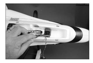
O 6. Use a small piece of hook and loop tape to mount the remote receiver in the front of the fuselage as shown. You will need to use a pin drill and 1/8-inch (3mm) drill bit to drill a hole for the antenna as shown.
