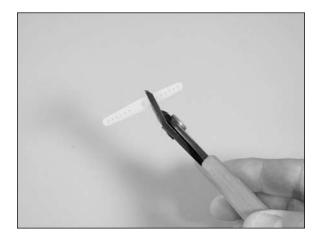
7. Use a pin drill and 5/64-inch (2mm) drill bit to enlarge the outer hole on the servo arm.
