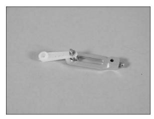
O 12. Remove the original servo arm from the servo using a #00 Phillips screwdriver. After centering the steering servo, install the long 3D arm prepared in the previous steps on the servo as shown.
