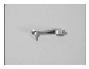
O 10. Use a #1 Phillips screwdriver to start the screw in to the outermost hole in the servo arm. Tighten the screw so the brass steering arm bushing is tight against the servo arm.
