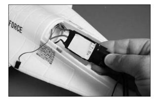
**Note**: Work through Step 3 before removing the backing from the hook and loop tape. Installation of the speed control can be tricky, and the stickiness of the hook and loop tape will make the installation even trickier. Keeping the backing on until ready will allow you to practice the installation of the speed control before your final performance.
