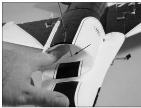
18. The nose gear will slide into the hole in the steering arm as its final destination. The screw at the steering arm will then be tightened so it is resting in the flat area as indicated back in Step 14. Use a #1 Phillips screwdriver to tighten the screw in the steering arm. Always remember to use threadlock on metal-to-metal fasteners to prevent them from vibrating loose.
