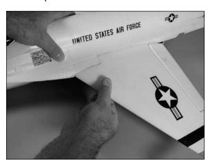
4. Fit the remaining wing panel to the fuselage. Stand 6-9 feet (2-3 meters) from the front of the airframe. When viewed from the front, both panels should be flat (parallel) along the bottom to be properly aligned. Use sandpaper to lightly sand the plastic joiner to correct the alignment.
