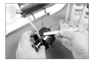
7. Insert the fan assembly into the fuselage, making sure to guide the wires into the notch in the fuselage. If not, the fan hatch will not fit correctly when it is time to install. Use low-tack tape to keep the fan held in position until the epoxy fully cures.
