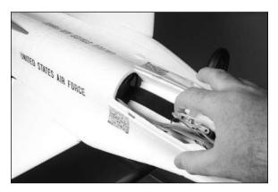
3. Place the battery into the battery compartment in the fuselage. The battery will be positioned in the compartment to achieve the correct Center of Gravity when you are using the recommended setup. The forward end of the battery should just clear the nose wheel steering arm.
