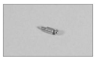
9. Slide the brass steering arm bushing through the slot in the steering arm. Note the direction of the screw in relationship to the steering arm.
