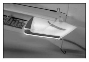
3. If the surface is not centered, use a pair of pliers and carefully lengthen or shorten the pushrod of that surface by bending the U shape in the pushrod.
