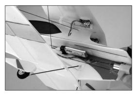
Note: The battery can be moved fore and aft to allow for the Center of Gravity adjustment. Start with the battery in the middle of the hook and loop strip. Adjust the battery forward or rearward to fine-tune the center of gravity.
