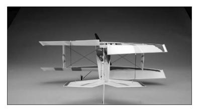
With the aileron stick pushed right, the right aileron should move up and the left aileron should move down.
