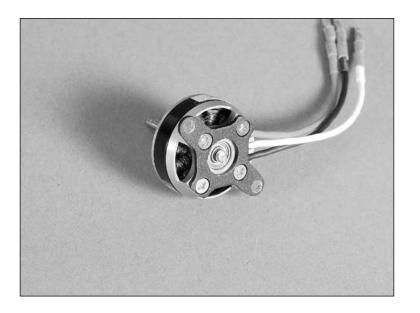
• 5. Attach the motor to the plywood mount using two #2 x 8mm wood screws or two #3 x 8mm wood screws.
