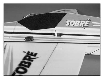
○ ○ 9. Locate the 4.5-inch (115mm) pushrod. Install the "Z" bend into the middle hole of the control horn that is one away from the aileron. Pass the pushrod through the connector. Check that the aileron servo is centered using the radio and parallel to the aileron hinge line. Hold the aileron parallel to the wing and use the 2mm x 4mm screw in the connector to secure the pushrod wire. Repeat for the other aileron pushrod.
