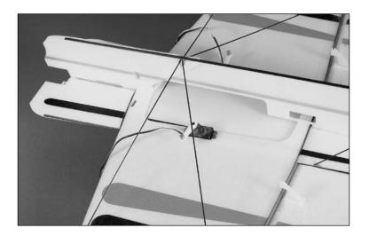
*Note*: Position the aileron servo arm parallel to the aileron hinge line.
