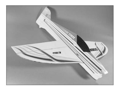
*Hint*: Fold one of the ailerons up and onto the wing to make it a little narrower to install into the fuselage. Push the wing past center to move the aileron back into position, then center the wing.
