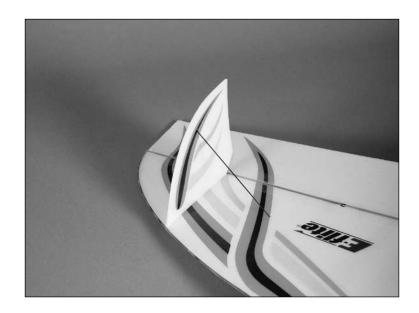
Glue the bottom SFG into position. Glue the 4.3-inch (110mm) carbon rod to the SFG. Check that the top and bottom SFGs are still perpendicular to the wing. Use Foam-compatible CA to glue the carbon rods to each other and to the wing.
