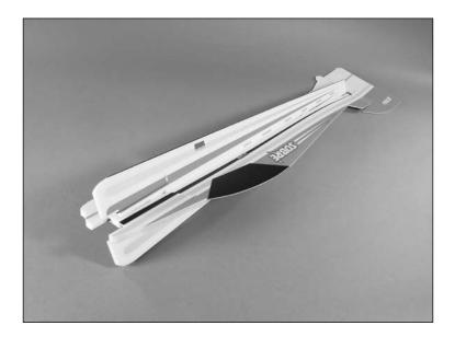
2. Locate the wing and slide it into the vertical fuselage underneath the horizontal fuselage. Use care not to damage either the vertical or horizontal fuselage pieces.
