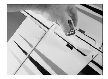
*Hint*: Use the holes for the aileron servos to aid in the alignment between the horizontal fuselage and wing.
