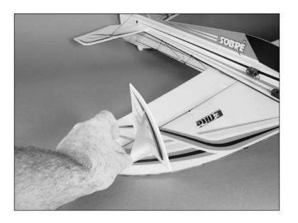
2. Locate a 4.3-inch (110mm) carbon rod. Position the rod in the predrilled holes in the SFG and wing. Use foam-compatible CA to glue the carbon rod to the SFG ONLY at this time.
