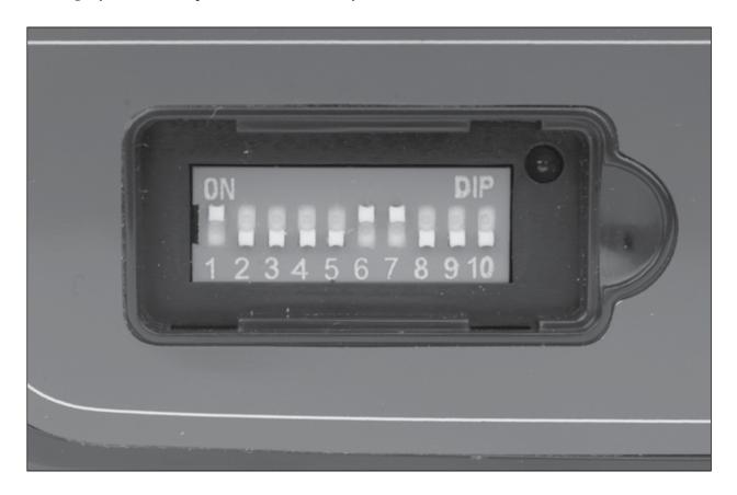
If the controls still do not respond properly after ensuring that the servo reversing dip switch positions are correct, you may also check the servo connections on the receiver side of the 4-in-1 unit. These should be positioned as follows (when viewing the helicopter from behind):
