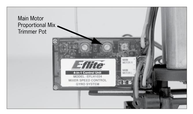
• In a stable hover, with the rudder trim centered and no rudder control input, note toward which direction the nose of the helicopter is trying to drift. If the nose of the helicopter is drifting to the left, you will want to increase power to the right-hand motor (spinning the upper main rotor blade). This is accomplished by turning the "proportional" trimmer pot clockwise. (+)
