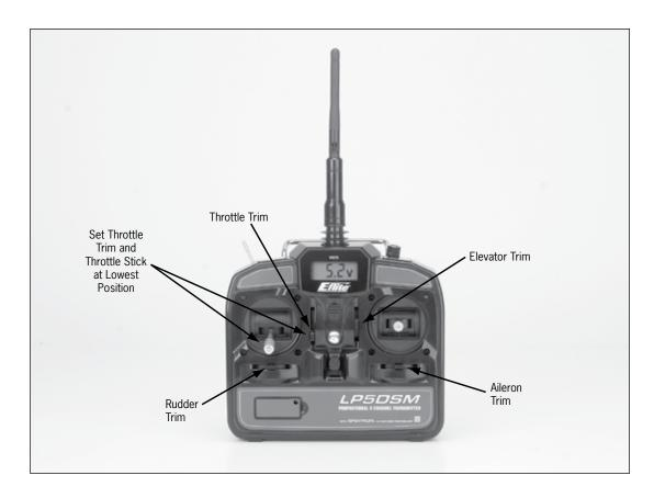
After confirming that the transmitter has been turned on and has an adequate level of battery power as displayed by the LCD screen at the top of the transmitter, it is now safe to connect the flight battery to the 4-in-1 unit.
