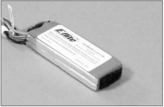
The battery can be installed through the opening in the rear of the body. Be sure to install the end of the battery with the loop material first. If you have installed the loop material on the end of the battery with the wire leads, be sure that the wire leads are oriented to the left side of the model so that they can pass by the stop. Slide the battery into the support frame until the hook and loop material makes contact.
