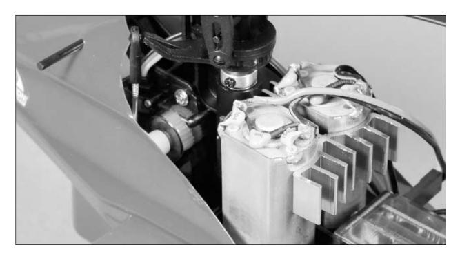
The main motor heat sink is now installed and ready for flight.
