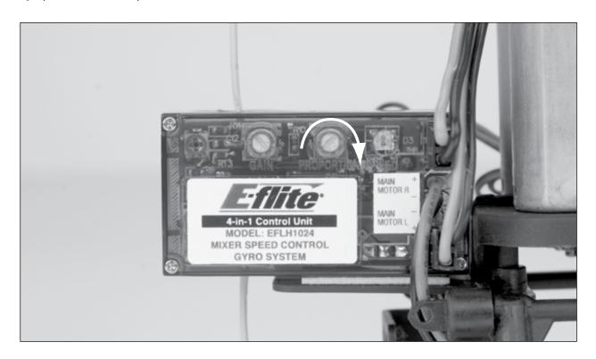
• If the nose of the helicopter is drifting to the right in hover, you will want to increase the power to the left-hand motor (spinning the lower main rotor blade). This is accomplished by turning the "proportional" trimmer pot counterclockwise. (–)
