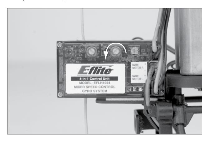
Note: You must always power down the 4-in-1 unit before making adjustments to the proportional mix trimmer pot. Any changes made to the trimmer pot will not take effect until the 4-in-1 unit is reinitialized and re-armed.
