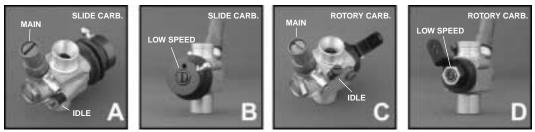
IMPORTANT: Carburetors are very sensitive to minor adjustments. Any adjustments should be made in increments of 1/16th to 1/8th of-a-turn, at a time. New carburetors should be set to the following guidelines and are <u>not</u> considered pre-set from the factory.
