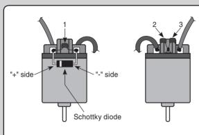
Motors with no suppressor capacitors, or inadequate suppression, may cause the MC800C Ver.2 to malfunction. Always solder the capacitors supplied to your motor.
