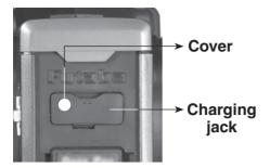
When charging the NT8F700B Ni-cad battery with the special charger, allow about 15 hours for charging. If the transmitter has not been used for some time, cycle the battery by charging and discharging it two or three times.
