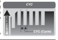
The smaller the set value, the faster the pulse speed.
