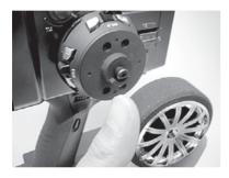
**3** Remove the 4 steering wheel unit cover screws.
