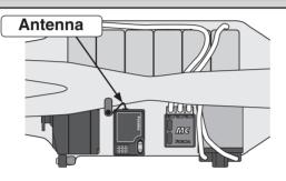
Install the receiver as far away from battery, motor controller, motor, silicon cord and other noise sources. Keep it away from the antenna wire, in particular.
