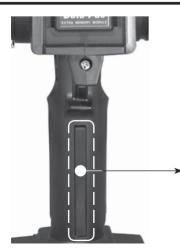
A vibrator is built into the grip of the T3PKS. The vibrator vibrates at racing timer lap navigation, time-up, and low battery alarm. (p.104)
