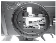
**3** At the opposite side, connect the steering wheel unit connector and Install the steering wheel unit, steering wheel cover, and wheel to their original positions.
