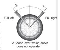
and right. Therefore, set the RIGH and LEFT value by checking servo operation.
