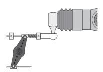
Adjust the throttle servo so that unreasonable force is not applied when the engine carburetor is full open, full close, and the brakes are applied fully.
