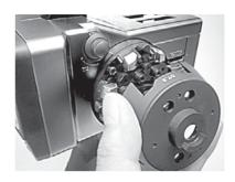
**5** Remove the 4 steering wheel screws.
