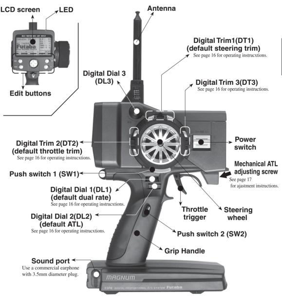
\*The switches, dial, and trimmers in the figure are shown in the initial setting position.
