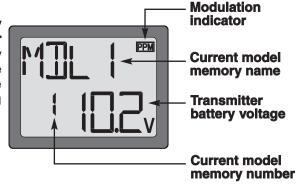
**Note**: Feel free to explore by scrolling through the programs and viewing the displays using the MODE and SELECT keys. The MODE and SELECT keys only determine what will be displayed on the screen and will not change any of the settings. Only when using the DATA INPUT lever will you be able to change any of the settings.
