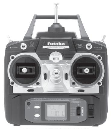
INSTRUCTION MUNUAL for Futaba 6EXHP 6-channel, PCM/PPM(FM) selectable Radio control system for helicopter
