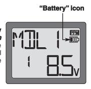
**Note**: When the transmitter voltage reads **8.9 Volts** you will still have approximately ten minutes (or less) before losing operational range, so this is the recommended **absolute minimum** voltage. If the transmitter ever reaches 8.9 Volts, land as soon as safely possible. A more reasonable margin of safety would be to quit flying for the day (or recharge the batteries) when the transmitter battery.
