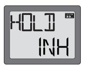
Push the DATA INPUT lever upward. This will cause the flashing "INH" display to change to a flashing "ON" display. Now the "HOLD" function is on.
