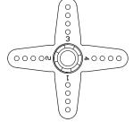
To center the servos, connect them to the receiver and turn on the transmitter and receiver. Center the trims on the transmitter, then find the arm that will be perpendicular to the pushrod when placed on the servo.
