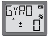
Flip the gyro (CH5) switch up and down. This will cause the arrow points up and down on the display simultaneously with switching operation and show the position of the switch. Push up or down DATA INPUT lever to set the gyro gains both switch up and down position. Gyro gain can be adjust from -100% to +100%.
