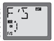
Carry out similar procedure like this in setting "F/S" function for other channels. Use Mode key to show a channel and do the same. But, CH3 (throttle) is set to 20% of the full throttle for "F/S" function as a default.
