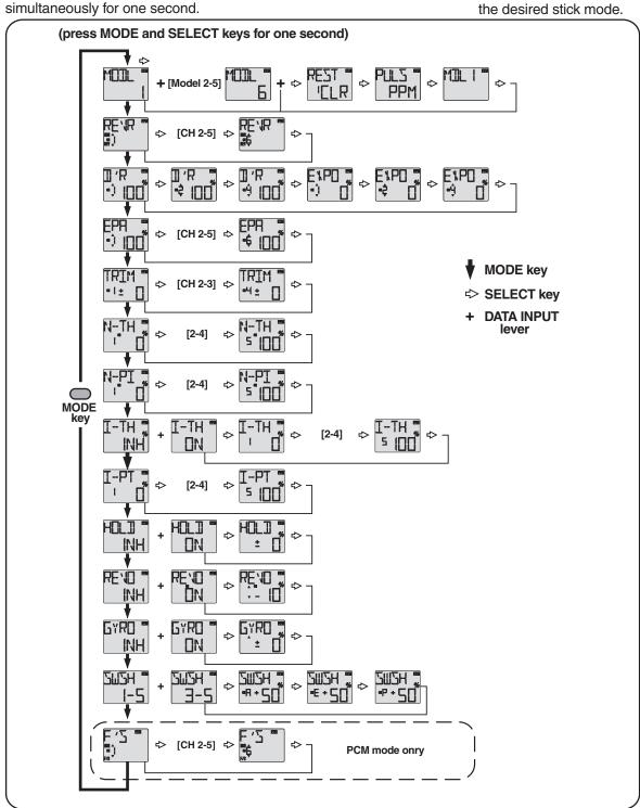
Simultaneously Press the "MODE" and "SELECT" keys and hold them down for one second to enter the programming mode. Press the keys again (or turn off the transmitter) to exit the programming mode.
