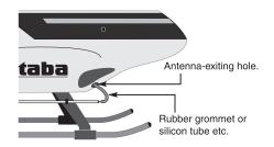
Place the receiver antenna out from the fuselage part to the nonmetal tube installed in skid etc. Please keep antenna away from parts that made of metal and carbon graphite.
