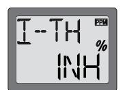
2. Push the DATA INPUT lever upward. This will cause the flashing **"INH"** display to change to a flashing **"ON"** display. Now the I-TH function is on. Push the SELECT key, throttle stick position number will appears on left side of display and "%" is blinks.
