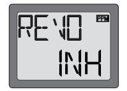
2. Push the DATA INPUT lever upward. This will cause the flashing "INH" display to change to a flashing "ON" display. Now the "REVO" function is on.
