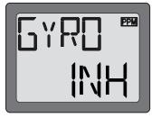
4. Push the DATA INPUT lever upward. This will cause the flashing "INH" display to change to a flashing "ON" display. Now the mixing is on.
