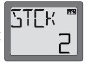
To change the mode, simultaneously depress the MODE and SELECT keys, then turn on the power. The current mode will appear on the LCD screen. Push the DATA INPUT lever up or down to change the mode. If a mode is selected that moves the throttle control to the right stick, **the throttle detent mechanism will have to be moved as well.** This can be done by the Futaba Service Center. (See page 2)
