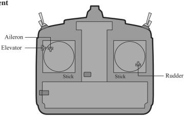
Mode 2 transmitter with rear cover removed.
