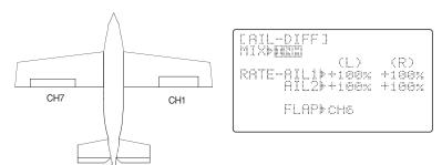
Aileron differential is primarily used on 3 or 4-servo wings, with one servo(s) operating inboard flap(s) on CH6 or CH5 & CH6, and All-DIFF controlling proper aileron operation of 2 aileron servos, plugged into CH1 and CH7. The ailerons can not be moved like flaps when using All-DIFF, except if using AIRBRAKE (see p. 55.) (Note that even if you make FLAP-TRIM active while using All-DIFF, it will not have any effect. ONLY AIRBRAKE controls the ailerons as flaps in the All-DIFF configuration.)
