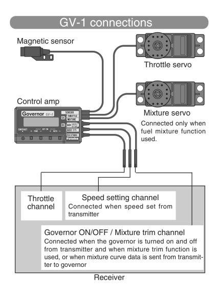
What is a governor? A governor is made up of a set of sensors which read the RPM of the helicopter's head, and a control unit that automatically adjusts the throttle setting to maintain a constant head speed regardless of changes in pitch of blades, weather conditions, etc. Governors are extremely popular in competition helicopters due to the consistency provided.
