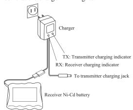
The initial charge, and any charge after a complete discharge, should be at least 18 hours to ensure full charge. The batteries should be left on charge for about 15 hours when recharging the standard NR-4J, NR4F1500 and NT8S700B Ni-Cd batteries.
