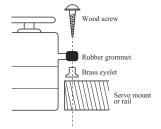
① Use the supplied rubber grommets when you mount each servo. Be sure not to over-tighten the screws. If any portion of the servo case directly contacts the fuselage or the servo rails, the rubber grommets will not dampen the vibration, which can cause mechanical wear and servo failure.
