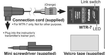
• Use the miniature screwdriver supplied to operate the Link switch.
