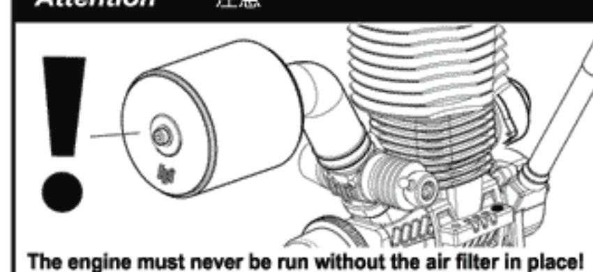
The engine must never be run without the air filter in place!
