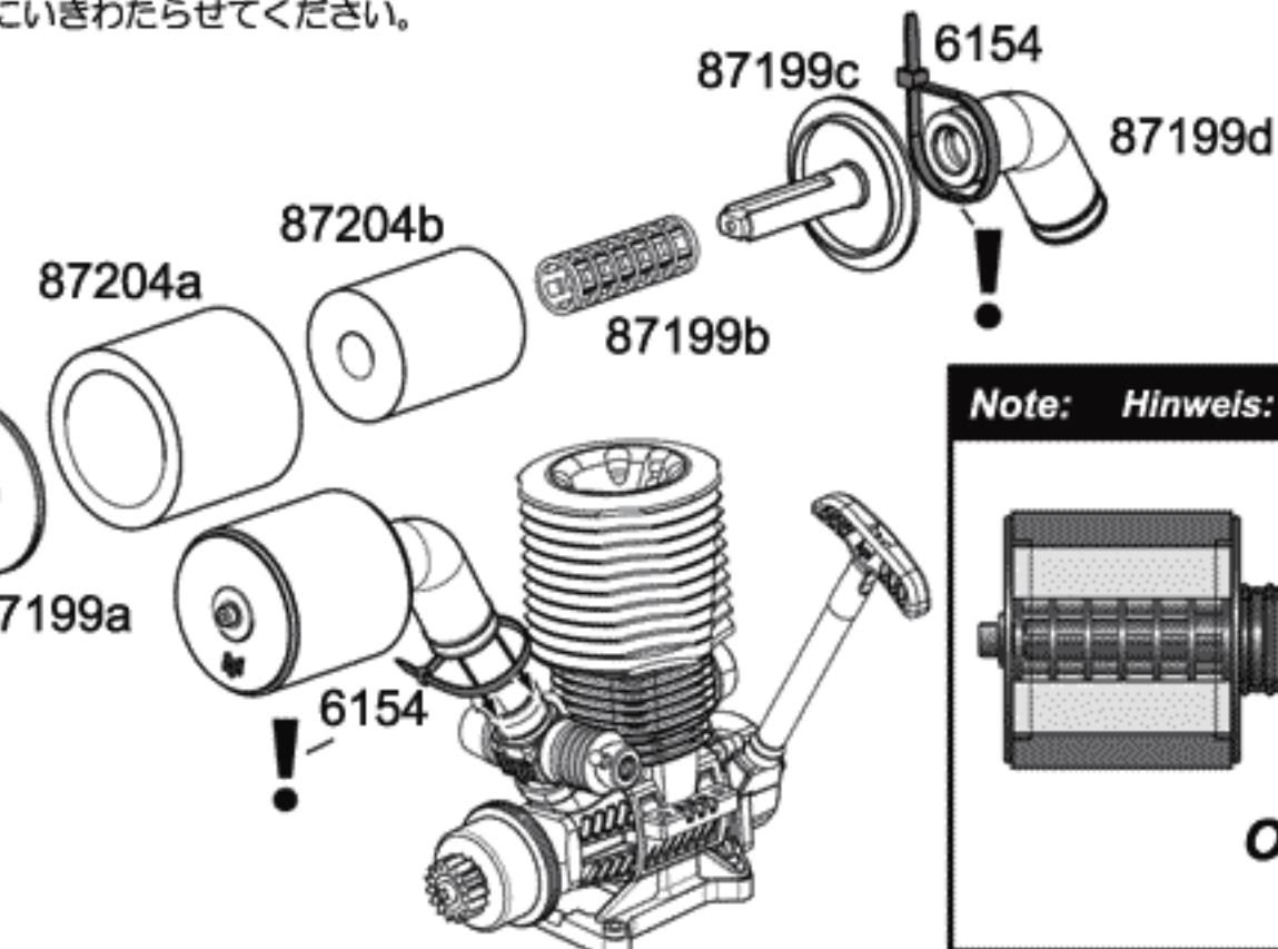
**Reinstalling The Air Filter:**
