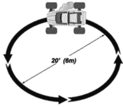
Place the vehicle on the ground. The vehicle should not move when idling. If it does, adjust the trim setting on the transmitter so the vehicle does not move. Drive the vehicle in a 20 foot (6m) oval applying throttle (below 1/2 throttle), coast for a short period of time to allow the engine to cool, then accelerate again. Continue this process for a total of two tanks of fuel.
