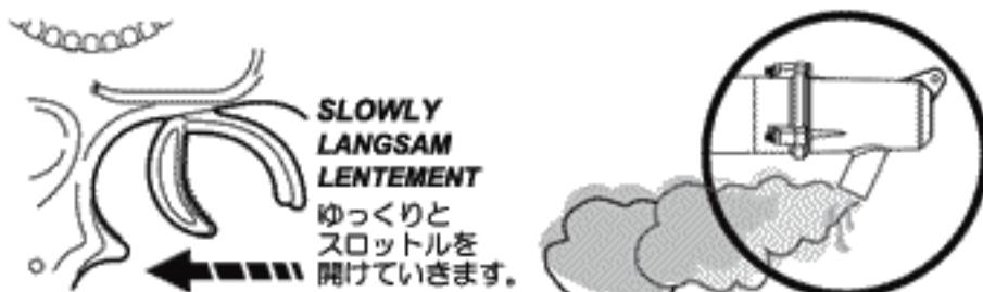
Turn on the transmitter and receiver, re-fill the fuel tank and follow the starting procedures in steps 1-5. With the tires off the ground, use the radio to slowly increase the throttle until it reaches full speed, then release. This will help clean the excess oil out of the engine. Because of the rich break-in settings, the motor needs to periodically be "cleaned out" to prevent it from stalling.
