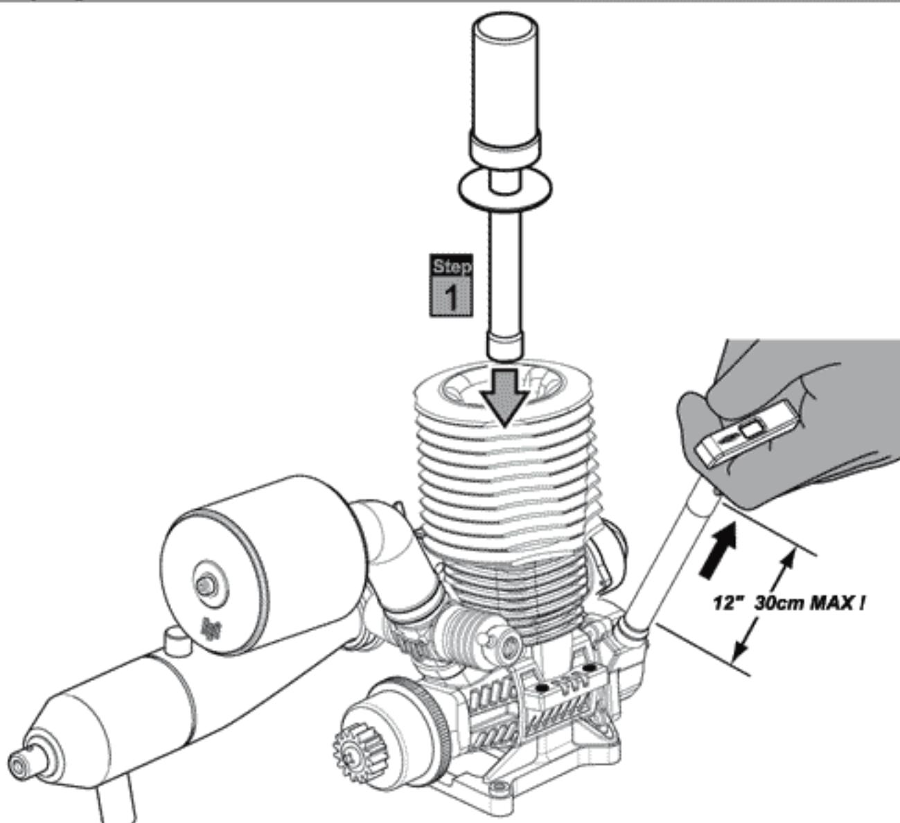
Attach the glow igniter to the glow plug. Start the engine by pulling the starter chord in short pulls (no longer than 30cm max). Adjust the throttle servo so the engine runs fast enough to idle smoothly without engaging the clutch or turning the wheels. Remove the glow igniter as soon as the engine is running. Run the engine for one tank of gas. If the motor shuts off, repeat steps 1-4.
