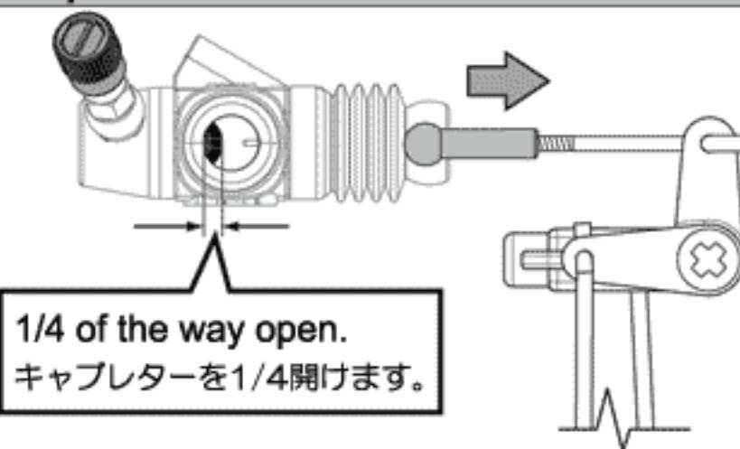
Make sure the receiver switch is off. Manually turn the throttle servo by hand until the carburetor is 1/4 of the way open.
