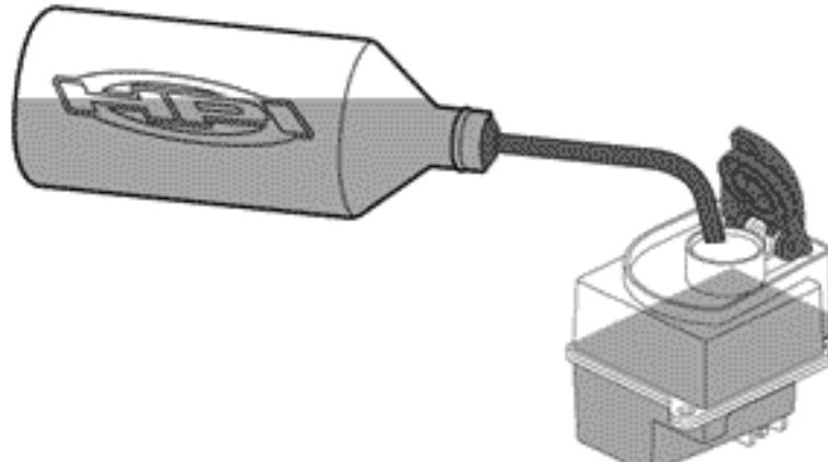
Fill the tank completely with fuel. Use only 20 to 25% Nitro content fuel. Use high quality branded model car fuel only. Using the non-car fuels could void your warranty.
