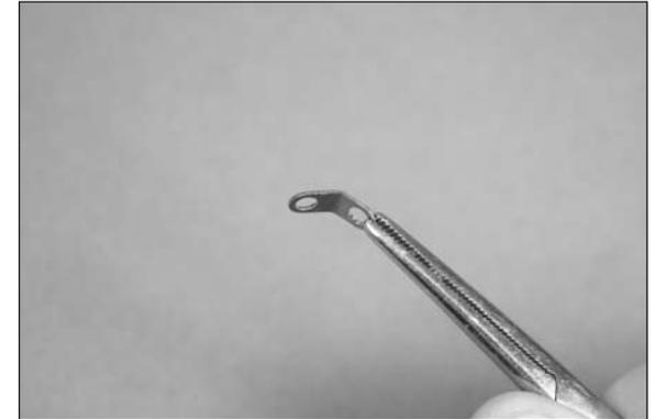
□□ 8. The shorter strut can now be attached to the stabilizer using a 4-40 x 5/8-inch button head cap screw, #4 washer, 4-40 lock nut and the brass tab. Make sure the washer is between the stabilizer and brass tab to space the tab slightly away from the structure. Leave the hardware loose so the struts can be positioned. When installing the top wire strut.
