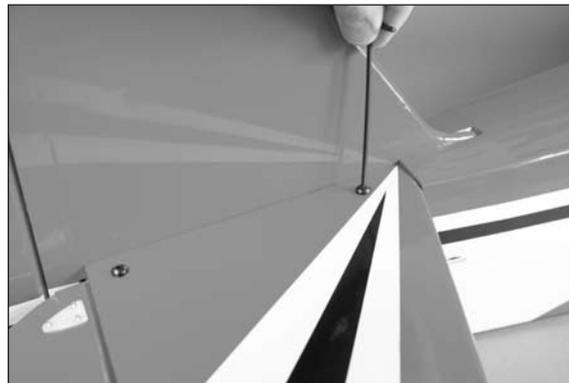
**Hint:** A machined hex wrench is helpful to allow the bolts to be tightened and not strip the head of the bolt.
