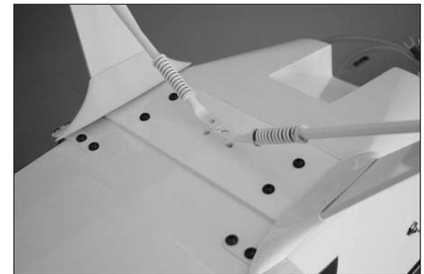
**Hint:** A machined hex wrench is helpful to allow the bolts to be tightened and not strip the head of the bolt.
