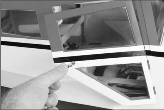
2. Connect the charger lead to the connection at the charge jack. The model includes a 2700mAh 5-cell Nickel-Metal Hydride (Ni-MH) battery. Be sure and use a good quality charger. We recommend to cycle the receiver battery 2–3 times prior to flying.
