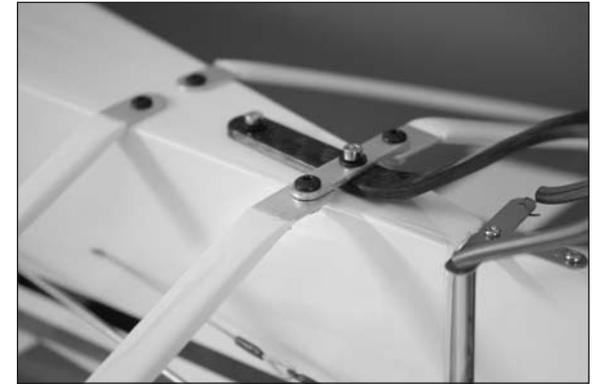
□□ 7. Use needle nose pliers to bend the brass tab at about a 30-degree angle.
