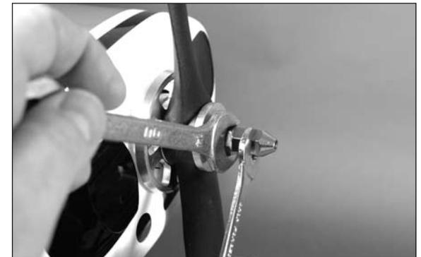
□ 9. The spinner can now be attached using the screw provided and a 4mm hex wrench. Make sure the spinner does not contact the propeller when it is installed.
