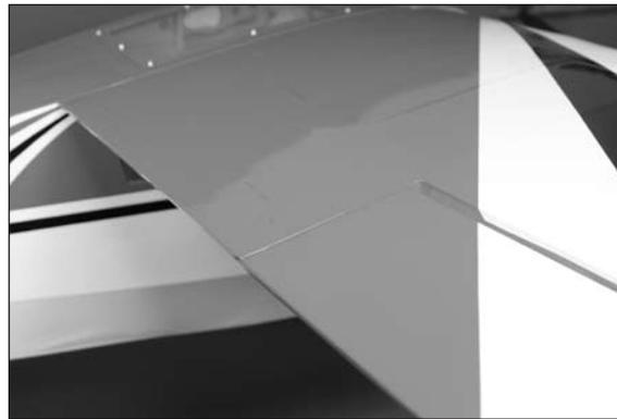
□ 7. Repeat steps 2 through 6 to attach the remaining wing panel and adjust the aileron.
