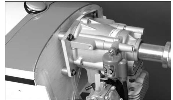
□ 3. Use side cutters to cut the tie-wrap holding the ignition ground leads and fuel tubing together.
