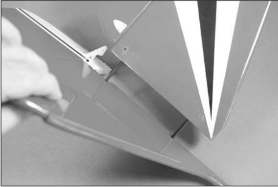
4. Slide the remaining stabilizer half into position. Press the stabilizer halves so they fit tightly against the fin as shown.
