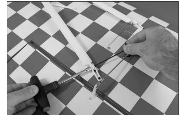
**Note:** Do not over-tighten the hardware that secures the wing struts to the fittings so the struts can be folded in for transport.
