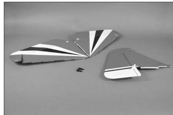
□ 2. Check that the hinges are glued securely by gently separating the control surface from the fixed surface. If any loose hinges are found, apply thin CA to both sides of the hinge. Allow the CA to soak into the hinge before checking them again.
