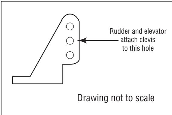
4. When connecting the clevises to the rudder, make sure there is a light amount of tension on the cables so the rudder has no play at neutral so it will not flutter.
