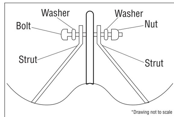
□ 14. Repeat steps 10 through 13 for the remaining top wire. Once both wires are set to length, use a 4-40 x 5/8-inch button head cap screw, two #4 washers and a 4-40 lock nut to secure the top wires to the fin.
