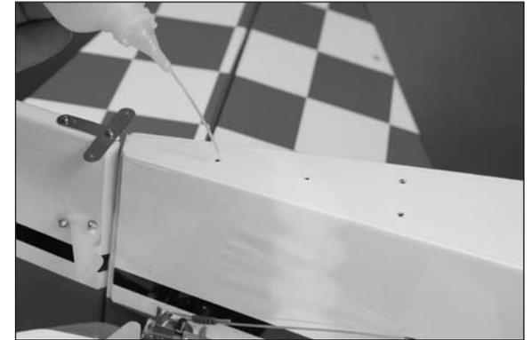
8. Attach the tail wheel assembly and the aluminum spreader tab on the fuselage using two 3mm x 15mm socket head wood screws and two 3mm washers. Tighten the screws using a 2.5mm hex wrench.
