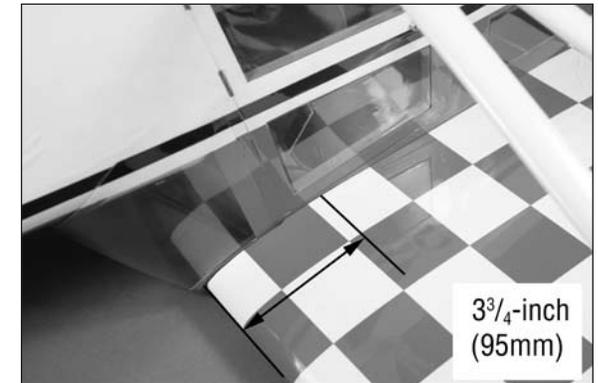
2. When balancing your model, make sure it is assembled and ready for flight with the fuel tank empty. Support the plane upright at the marks made on the wing with your fingers or a commercially available balancing stand. This is the correct balance point for your model.
