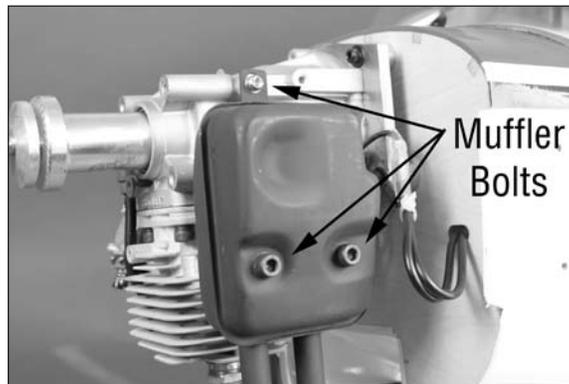
**Hint:** The use of high-temperature exhaust manifold sealant is helpful to help keep the manifold from leaking over time.
