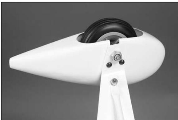
□ 5. With the landing gear fairing as close to the fuselage as possible, apply a small amount of silicone adhesive to the plywood inside the landing gear fairing. Slide the fairing tight against the fuselage and use low-tack tape to hold it in position until the adhesive cures. Gluing the fairing to the gear will allow the gear to be removed without damaging the fuselage.
