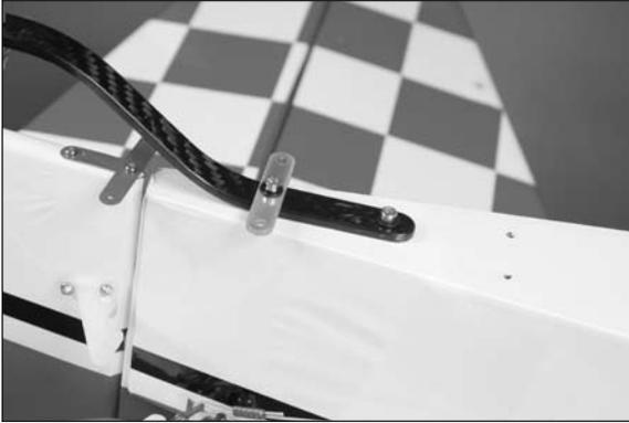
9. Connect the arm from the tail wheel to the tiller arm using two tail wheel steering springs. Make a loop on each end of the spring with needle nose pliers. Use care when bending the springs so the tail wheel is aligned with the rudder. Cut the excess spring using side cutters.
