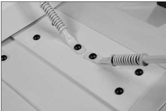
□ 4. Attach the wheel pants to the landing gear using four 4-40 x 1/2-inch button head cap screws and four #4 washers. Tighten the screws using 5/64-inch hex wrench.
