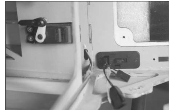
2. Follow the procedure as described in your radio manual for binding the receiver and transmitter. Check the operation of the rudder, elevator and throttle servos using the radio system.
