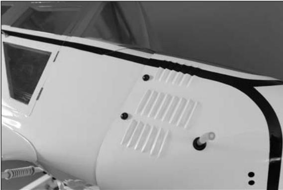
**Note:** The included velocity stack for the G26 is not being used as the carburetor is completely enclosed inside the cowling.
