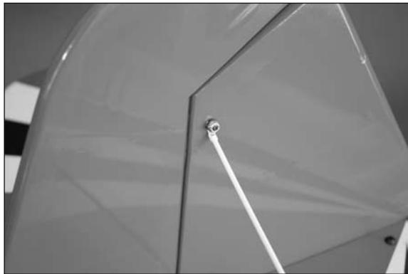
□ 15. Check the alignment of the fin to the stabilizer to make sure they are perpendicular to each other. Also check the alignment between the rudder and fuselage. If not, loosen the hardware slightly to adjust the alignment.
