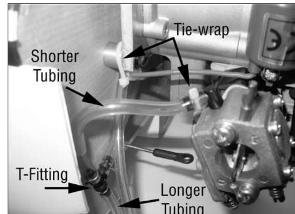
**Note:** Be sure and keep the fuel line and wiring away from the HOT exhaust muffler.
