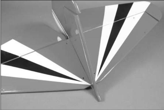
5. Remove the packaging from the tail of the fuselage. Place the assembly on the fuselage. The fin will fit into the slot along the top of the fuselage.
