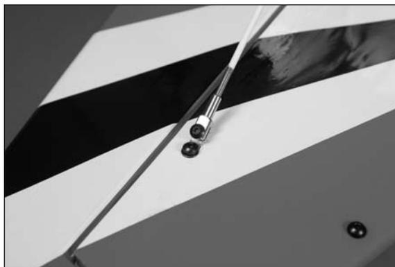
□□ 13. Adjust the length of the top wire so it just contacts the fin when positioned so the fin is 90 degrees to the stabilizer.
