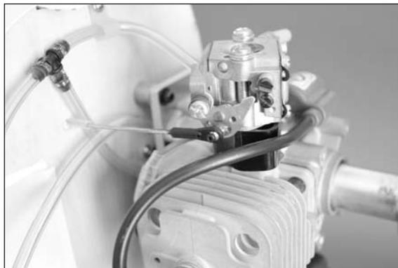
**Hint:** Remove the idle limit setscrew as you will adjust the idle from your transmitter using the throttle trim.
