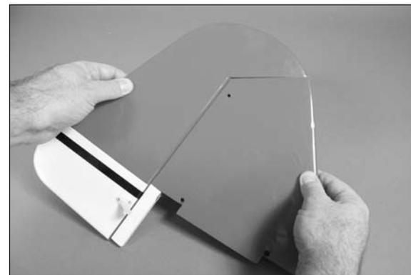
3. Separate the stabilizer halves. Slide the pins and one stabilizer half into the holes in the fin as shown.
