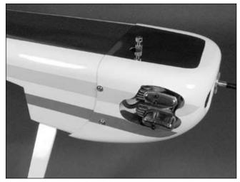
**Step 10** Attach the propeller and spinner onto the engine.
