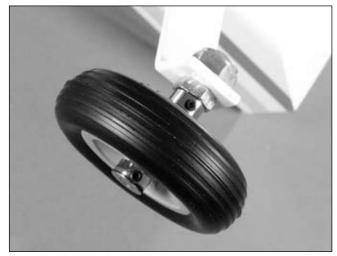
**Cool Tip**: Position the setscrews on the wheel collars facing directly down. This way you can get to them later to position the wheel on the axle.
