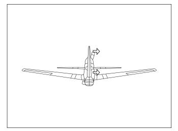
**Note**: Operating the functions at the transmitter opposite as described will result in the control surfaces moving opposite as well.
