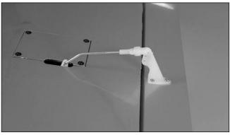
Connect the aileron servo leads as described in the previous section. Center the aileron trim on the transmitter.
