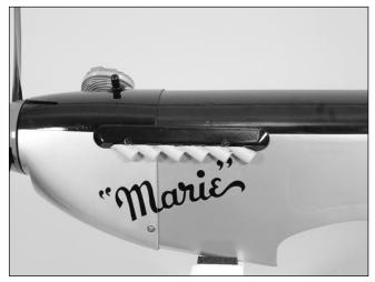
**Note**: The exhaust stack for the right side of the model is shorter than the left. This is necessary to clear the muffler.
