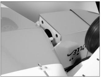
**Note**: Check to make sure the servo leads are inside the fuselage and not caught between the wing and fuselage.
