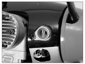
Move the throttle stick towards the top of the transmitter. The carburetor will now be in the fully open position.
