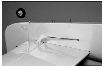
Center the trim lever for the elevator on the transmitter.
