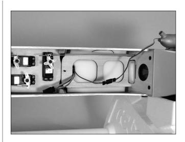
**Note**: There are two other leads that are for the aileron servos to plug into. The charger should not be connected to these plugs.
