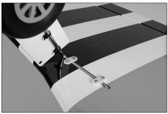
**Note**: Use care not to over-tighten the screws and damage the landing gear mount.
