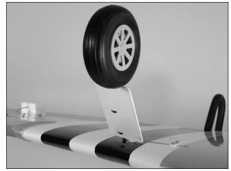
**Step 4** Repeat Steps 1 through 3 to install the right landing gear strut.
