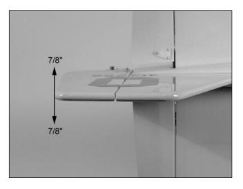
**Hint**: Place your ruler on a solid surface, rather than hold it in the air, to take measurements. This will guarantee your ruler is not moving. If the ruler is moving you will get inaccurate readings.
