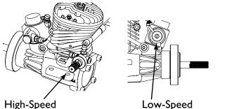
High-Speed Needle Adjustment Low-Speed Needle Adjustment
