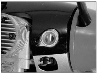
Move the trim lever up towards the top of the transmitter. The barrel in the carburetor should have an opening of around 1/16".
