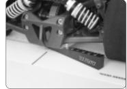
**Ride height:** The HUDY Ride Height Gauge part number #10 7713 or #107715 accurately checks the ride height front and rear, left and right. It is versatile enough to be used on all types of cars.
