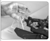
Remove the wheels from your car, and open front the one-way if available. Now, in place of the car wheels, mount each of the four wheel plates. If your axles use quick-release levers, please use a file or emery board to round the edges of the levers. This will make installation of the Set-Up stands easier and prevent damage to them.
