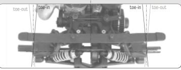
response, and a marginal decrease in top speed. Rear toe-out is not recommended. Front: With front toe-in, most cars will have less steering, and will actually steer in the turn a lot smoother. Front toe-out results in a more aggressive steering when entering the turn. However it can also cause the car to wander slightly in high-speed straightaways.
