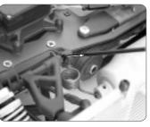
The Hudy Set-Up allows you to adjust caster with unmatched ease. Just position the front wheel plates on the front axles and read the angle on the gauges between the imaginary line that goes from the top articulation point of the spindle/C-hub to the bottom one, and the vertical line on the plate.
