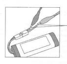
The connector wires must be different length, this would help prevent short circuit.
