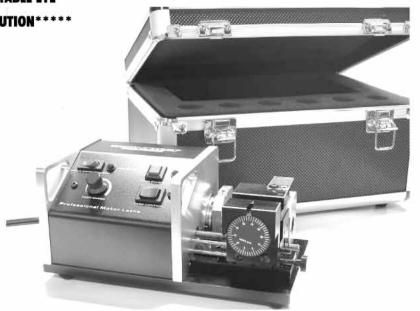
The gib adjustment for the carriage is located on the front of the lathe and below the cross-slide. The carriage should be adjusted so that it is free of play, yet guides smoothly so you get a clean, even cut on your commutators. These adjustments will be properly set from the factory, but you must fine-tune the adjustments as the gibs wear with use.
