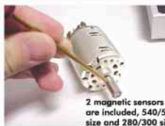
4. Install the correct size magnetic sensor
